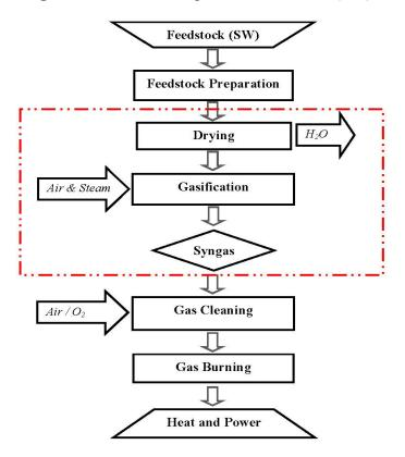
Figure 2. Schematic diagram of solid waste (SW).
