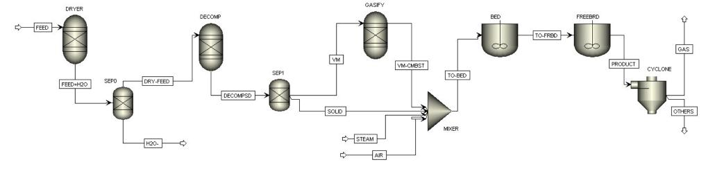
Figure 4. Advanced System for Process ENgineering (Aspen) Plus simulation flowsheet.
