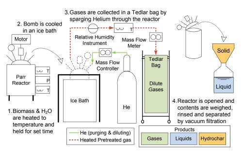
Figure 8. Flow diagram of HTC process and product collection.
