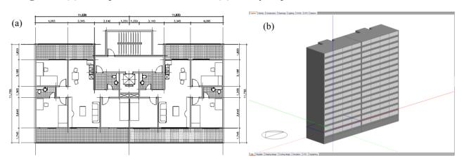
Figure 2. (a) Floor plan for the simulation; (b) flat style apartment model with fifteen stories.
