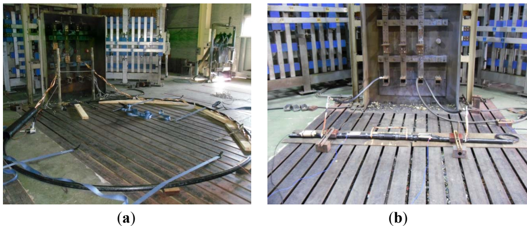
Figure 9. Short-circuit test: (a) OFCPC and (b) cable joint.
