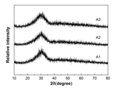
Figure 1. XRD results of the pre-melted slags.
