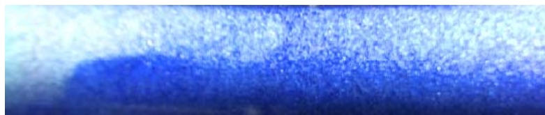
Figure 10. The picture shows water (white color) override at the top of the formed gel (blue color) in the middle of the sand-pack A. The injected slug size of Na-silicate (5 wt% at pH = 10.42) is 0.5 PV.
