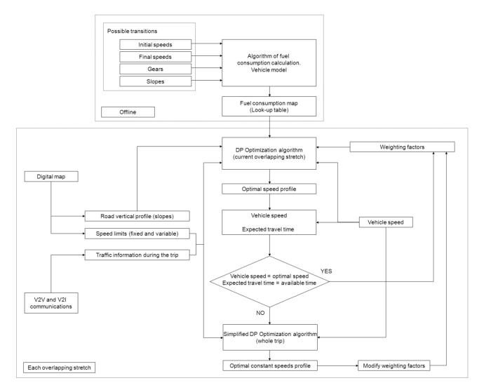
Figure 1. Scheme of the optimization process.
