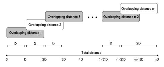
Figure 2. Overlap of the partial speed profiles.
