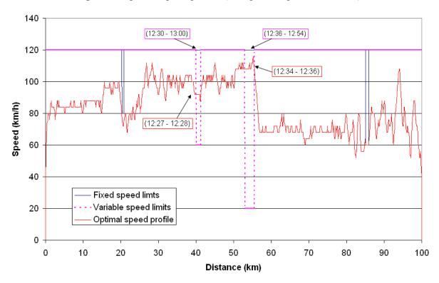
Figure 7. Optimal speed profile (unexpected speed restriction).
