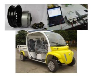
Figure 9. In-wheel motor, dSPACE and prototype EV.
