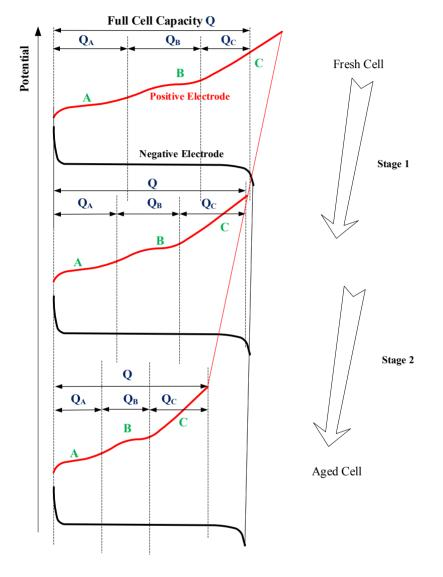
Figure 8. Schematic of the two stage capacity fade mechanism.
