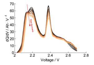
As shown in Figure 6, before 630 cycles, with increased cycle number, the IC curves in the Region C increase, and after 630 cycles, the IC curve decreases. There is no clear resistance increase since the position of all the peaks hardly changes.
