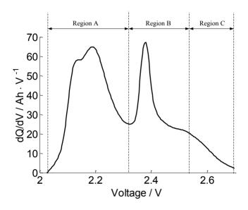
Figure 4. The incremental capacity (IC) curves of new Cell A.
