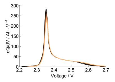
Figure 11. The high voltage region of IC curves of Cell B after every 90 cycles: (a) after 0 cycles up to 810 cycles; and (b) after 810 cycles up to 1080 cycles.
