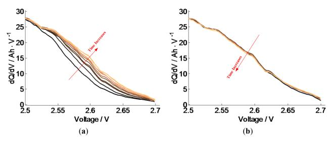
**Figure 12.** The IC curves of Cell C after every 90 cycles up to 1080 cycles; with cycle number increase, line color changes from black to tan.
