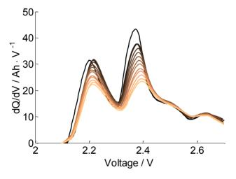
Figure 13. The high voltage region of IC curves of Cell C after every 90 cycles: (a) after 0 cycles up to 810 cycles; and (b) after 810 cycles up to 1080 cycles.
