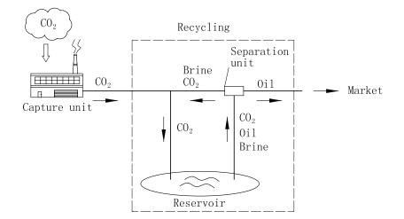
Figure 12. CO<sub>2</sub>-EOR system flow diagram.
