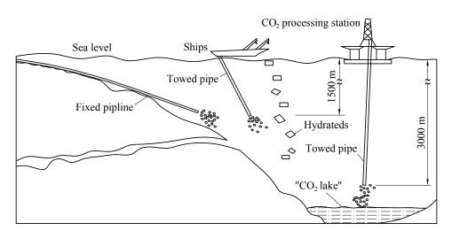
Figure 11. CO<sub>2</sub> storage in a deep sea schematic diagram.
