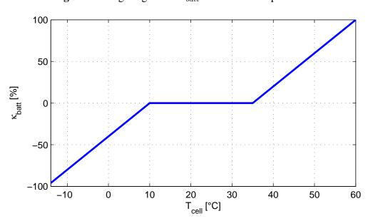
**Figure 4.** Weighting factor  $\kappa_{batt}$  versus cell temperature.
