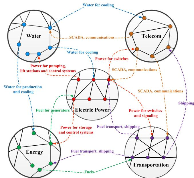
**Figure 1.** (Color online) Illustration of the interdependent relationship among different infrastructures [54]. These complex relationships are characterized by multiple connections between infrastructures, feed-back and feed-forward paths and intricate, branching topologies. The connections create an intricate web that can transmit shocks across multiple infrastructures. [54]. This figure is from Ref. [59].
