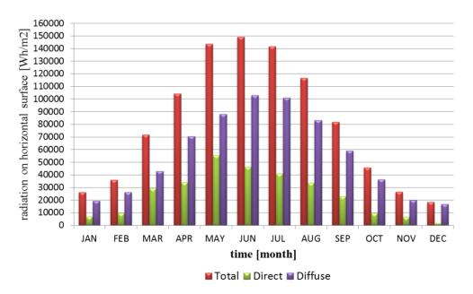
**Figure 2.** Distribution of solar radiation during the year including total, direct and diffuse components for the city of Poznan, based on [18].
