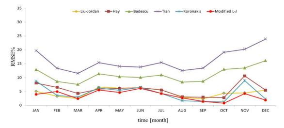
**Figure 3.** The differences in RMSE% of incident solar radiation of multiple models for a plane facing south at an inclination angle of 30° located in Poznań, Poland.
