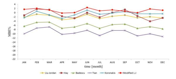
**Figure 4.** The differences in MBE% of incident solar radiation of multiple models for a plane facing south at an inclination angle of 30° located in Poznań, Poland.
