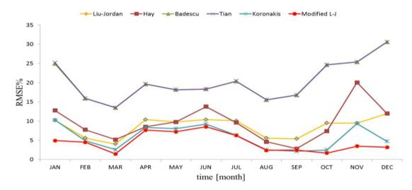
**Figure 5.** The differences in RMSE% of incident solar radiation of multiple models for a plane facing south at an inclination angle of 45° located in Poznań, Poland.
