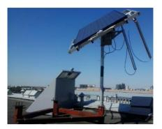
**Figure 1.** Two-axis tracking system with photovoltaic module, radiation power density meter and microinverter.
