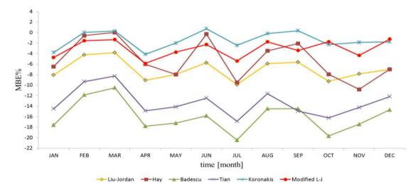
**Figure 8.** The differences in MBE% of incident solar radiation of multiple models for a plane facing south at an inclination angle of 60° located in Poznań, Poland.
