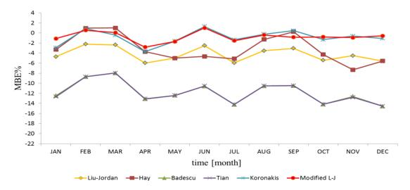
**Figure 6.** The differences in MBE% of incident solar radiation of multiple models for a plane facing south at an inclination angle of 45° located in Poznań, Poland.
