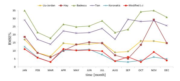
**Figure 7.** The differences in RMSE% of incident solar radiation of multiple models for a plane facing south at an inclination angle of 60° located in Poznań, Poland.
