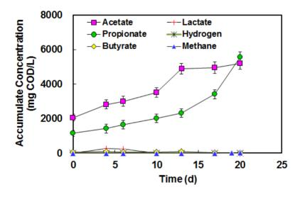
**Figure 6.** Profiles of organic acids and biogas in a batch mode fermenter using raw piggery waste and H<sub>2</sub> producing mixed culture (BA: 8.9 CaCO<sub>3</sub>/L, pH 8.7).
