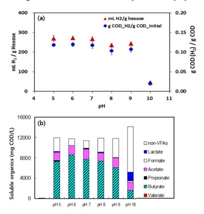
Figure 1. Hydrogen yield (a) and organic acids production (b) under designated pHs without BA supplementation (substrate: sucrose, initial COD = 16 g/L).
