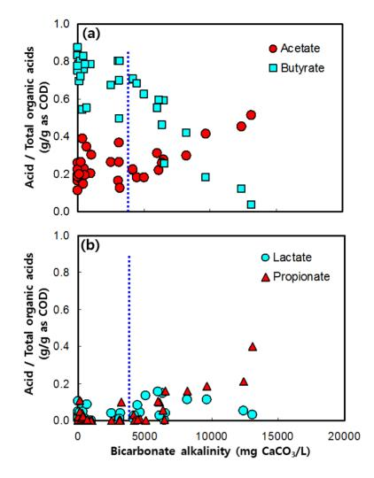
**Figure 5.** (a) Acetate and butyrate, (b) lactate and propionate in the batch hydrogen fermentation (substrate: sucrose) as a function of the BA.
