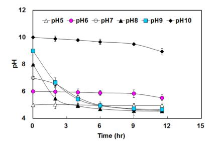
**Figure 2.** pH profiles during the batch biohydrogen fermentation (substrate: sucrose). Bicarbonate alkalinity was not amended.
