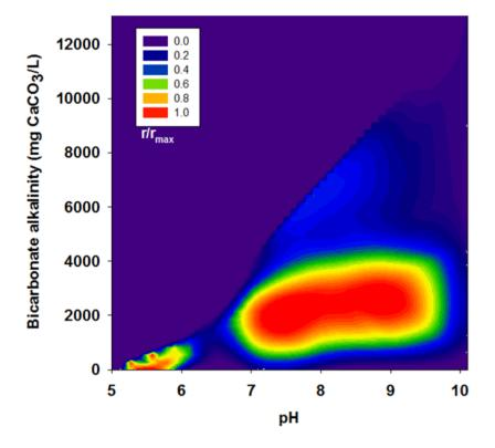
**Figure 4.** Hydrogen production rate of H<sub>2</sub> producing mixed culture with BA (substrate: sucrose). The  $r/r_{\text{max}}$  represents that specific hydrogen production rate (mL H<sub>2</sub>/g VSS-d) is divided by maximum hydrogen production activity.
