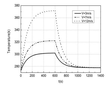
Figure 8. Thermal behaviour of the DFIG stator winding.
