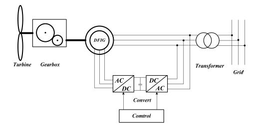
Figure 4. Configuration of a WT with DFIG.
