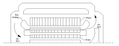
Figure 2. Sketch of the inner construction of a DFIG.
