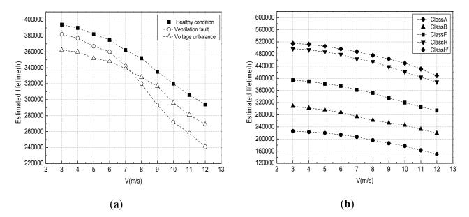
**Figure 15.** Lifetime downrating of stator windings subjected to generator system faults (**a**); lifetime estimation of stator windings with different Class ratings (**b**).
