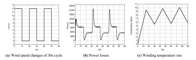
**Figure 10.** Power losses and temperature rise of stator windings for wind speed change with a 30 s cycle.
