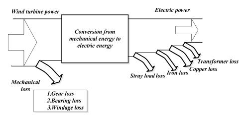
Figure 1. WT system power flow.
