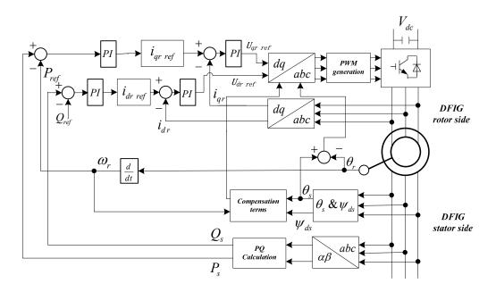
Figure 5. RSI-based stator flux vector control diagram.
