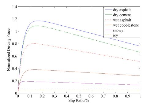
**Figure 5.**  $\mu$ - $\lambda$  curves of standard road conditions.
