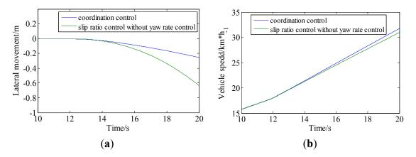
**Figure 17.** Comparison of experiment results of the proposed strategy and normal strategy on a low friction t road: (**a**) lateral movement and (**b**) acceleration performance.
