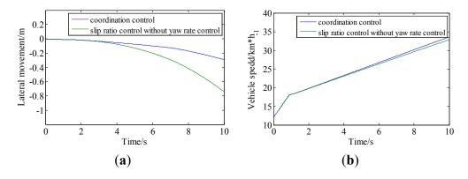
**Figure 11.** Comparison of simulation results of proposed strategy and normal strategy on variation friction coefficient road: (a) lateral movement and (b) acceleration performance.
