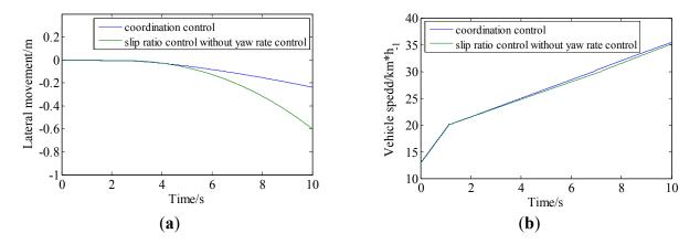
**Figure 13.** Comparison of simulation results of proposed strategy and normal strategy on variation split- $\mu$  road: (a) lateral movement and (b) acceleration performance.
