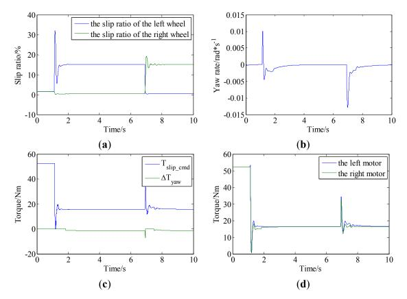
Figure 12. Simulation results of acceleration slip regulation on variation split- $\mu$  road: (a) slip ratios of driving wheels; (b) yaw rate of vehicle; (c) torque commands of slip ratio control and yaw rate control; and (d) motor torque outputs.
