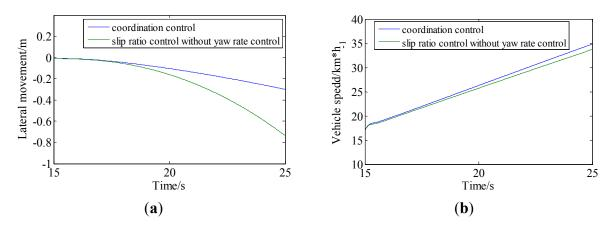
**Figure 19.** Comparison of experiment results of proposed strategy and normal strategy on variation friction coefficient road: (a) lateral movement and (b) acceleration performance.
