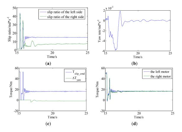
**Figure 18.** Experiment results of acceleration slip regulation on variation friction coefficient road: (a) slip ratios of driving wheels; (b) yaw rate of vehicle; (c) torque commands of slip ratio control and yaw rate control; and (d) motor torque outputs.
