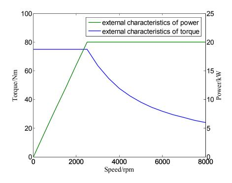
Figure 3. Motor power/moment external characteristics.
