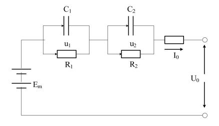
Figure 4. The equivalent circuit battery model.
