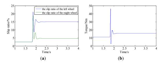
**Figure 6.** Typical slip ratio control progress without yaw rate compensation: (**a**) slip ratios of both wheels and (**b**) torque command.
