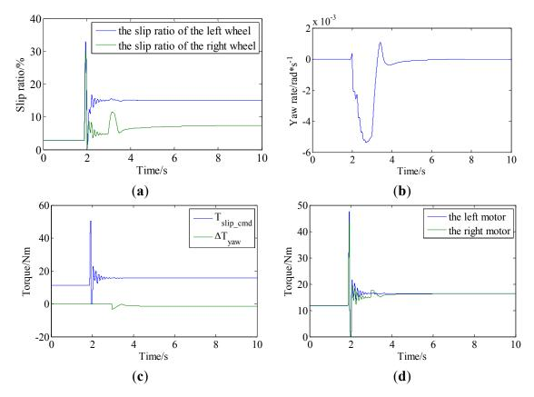
**Figure 8.** Simulation results of acceleration slip regulation on low friction road: (**a**) slip ratios of driving wheels; (**b**) yaw rate of vehicle; (**c**) torque commands of slip ratio control and yaw rate control; and (**d**) motor torque outputs.
