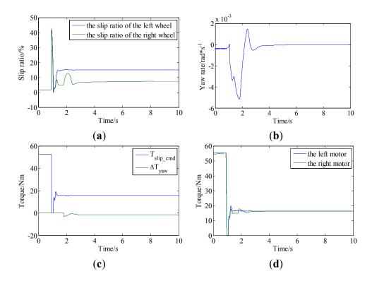
**Figure 10.** Simulation results of acceleration slip regulation on a varying friction coefficient road: (a) slip ratios of driving wheels; (b) yaw rate of vehicle; (c) torque commands of slip ratio control and yaw rate control; and (d) motor torque outputs.
