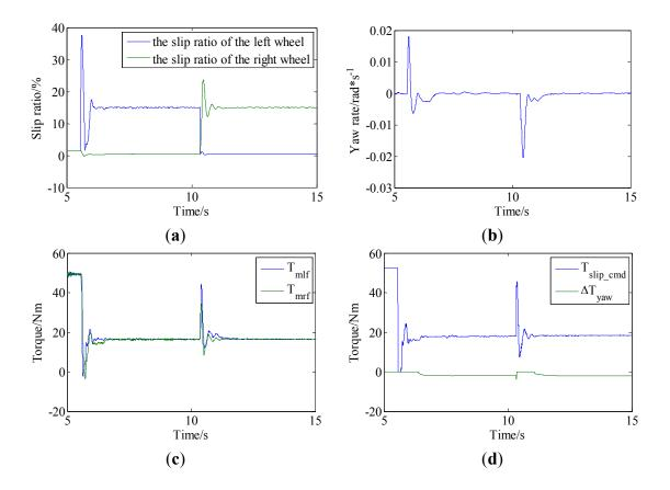
**Figure 20.** Experiment results of acceleration slip regulation on variation split- $\mu$  road: (a) slip ratios of driving wheels; (b) yaw rate of vehicle; (c) torque commands of slip ratio control and yaw rate control; and (d) motor torque outputs.
