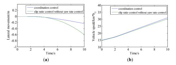
**Figure 9.** Comparison of simulation results of proposed strategy and normal strategy on low friction road: (a) lateral movement and (b) acceleration performance.
