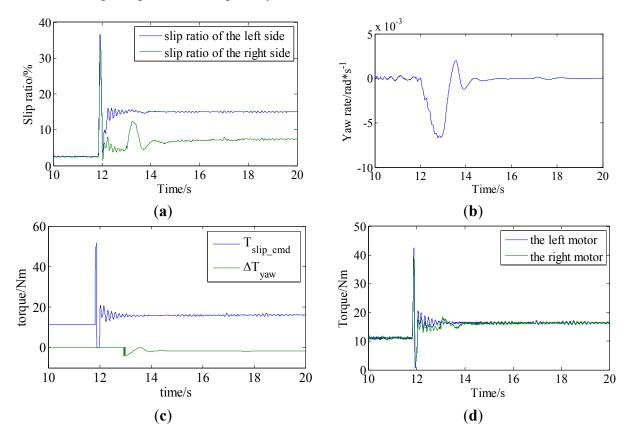
**Figure 16.** Experiment results of acceleration slip regulation on a low friction coefficient road: (a) slip ratios of driving wheels; (b) yaw rate of vehicle; (c) torque commands of slip ratio control and yaw rate control; and (d) motor torque outputs.
