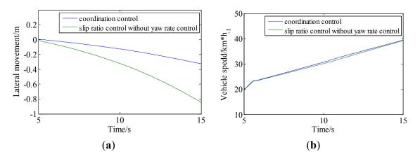
Figure 21. Comparison of the experimental results of the proposed strategy and normal strategy on a varying split- $\mu$  road: (a) lateral movement and (b) acceleration performance.
