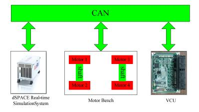
Figure 14. Structure of the test bench.
