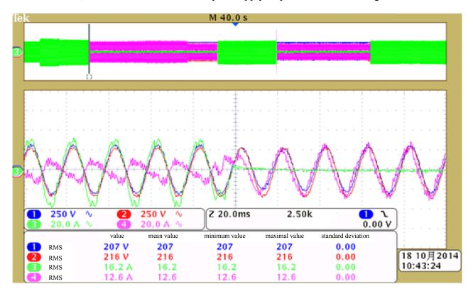
Figure 8. Conversion of the grid-connected mode to the autonomous mode.
