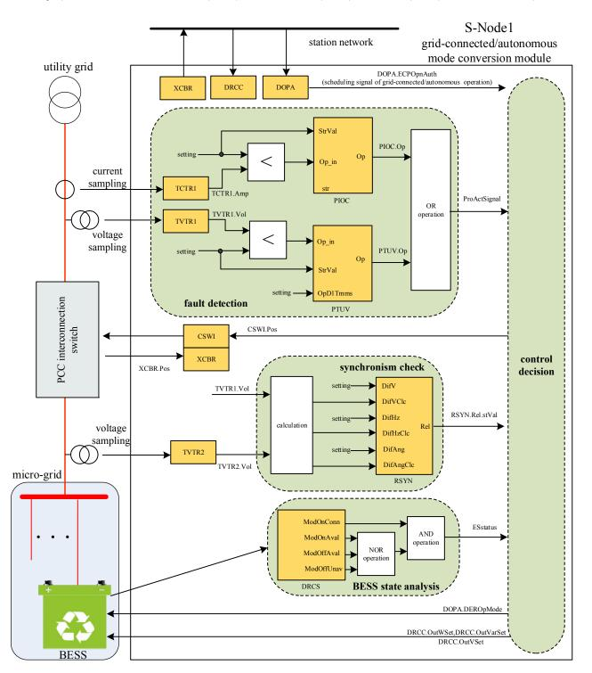
Figure 6. Procedures of grid-connected/autonomous mode conversion.
