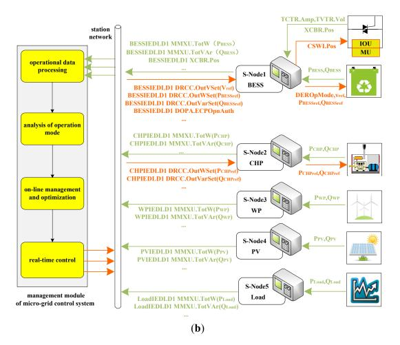
Figure 5. Data exchange in "plug and play" integration: (a) Data exchange for S-Node; (b) Data exchange for micro-grid.
