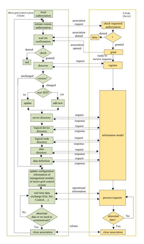
Figure 4. Procedures of "plug and play" integration.
