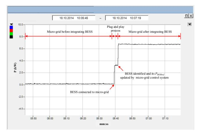
Figure 7. Power monitoring curves of BESS.
