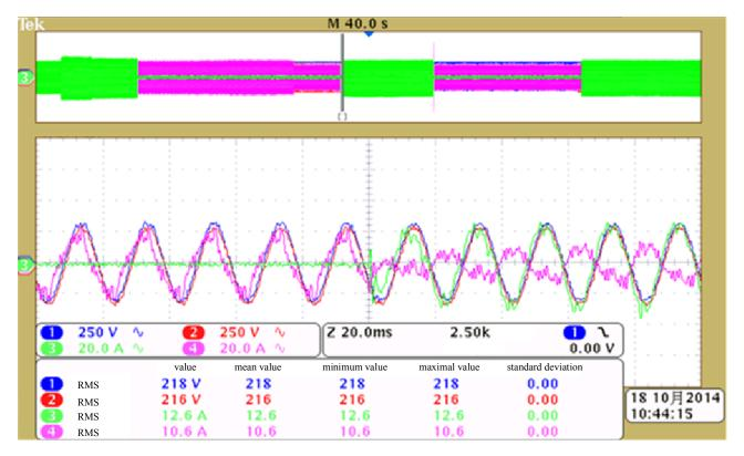
Figure 9. Conversion of the autonomous mode to the grid-connected mode.
