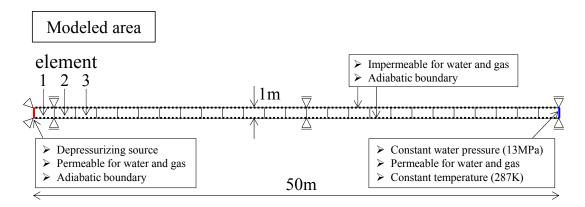
Figure 4. Simulation model and boundary conditions.
