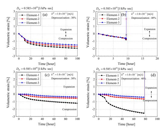
Figure 12. Time profiles of the volumetric strain  $\varepsilon_{\nu}$  (%). (a) Case-4-30; (b) Case-4-40; (c) Case-7-30; (d) Case-7-40.
