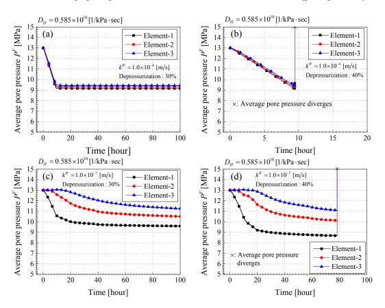
**Figure 10.** Time profiles of the average pore pressure  $P^F$  (MPa). (a) Case-4-30; (b) Case-4-40; (c) Case-7-30; (d) Case-7-40.
