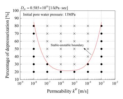
**Figure 7.** Stable and unstable regions of permeability and the depressurization level during the MH dissociation process.
