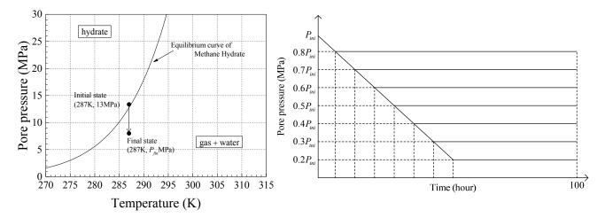
Figure 5. Conditions of change in pore pressure change at the depressurization source.
