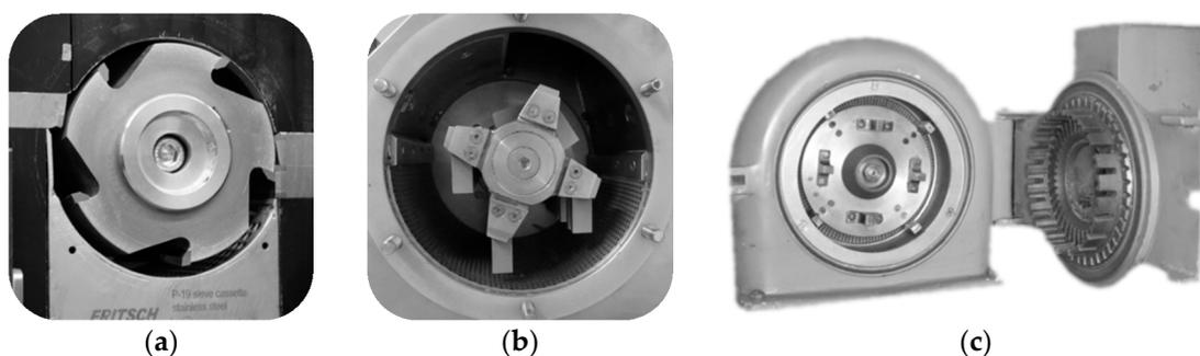
**Figure S2.** View of the grinding chamber of each of the three mills used. In (a) the blades of the CM, in (b) the flexible hammer elements of the HM and in (c) the geometry of the grinding ring inside the IM can be seen.
