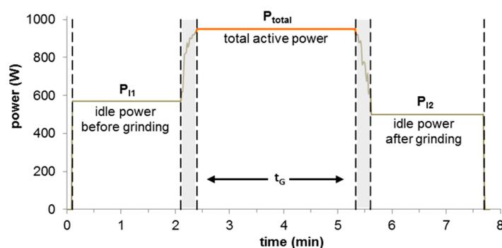
**Figure S3.** Typical power curve when recording the power consumption during grinding. Given are the defined parameters necessary for calculating the specific grinding energy.
