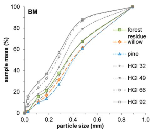
**Figure S4.** Cumulative particle size distribution obtained when using a ball mill (as prescribed in the HGI method) on three selected torrefied biomass pellets and four standardized HGI coals.
