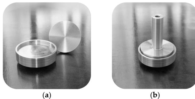
**Figure S1.** Picture of the anvil and plunger used during the hardness test: (a) Showing the two surfaces between which the pellets are compressed and (b) the plunger resting on the anvil without a pellet in-between them.
