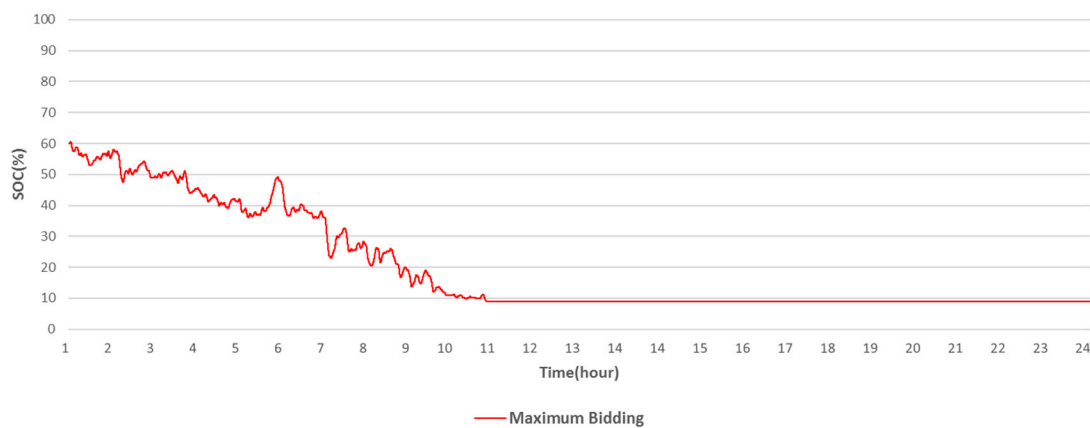
Figure 5. SOC of ESS in real-time operation simulation (Case 1—maximum bidding capacity plan).
