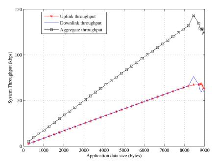
Figure 9. System throughput as a function of application data size.
