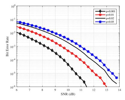
Figure 13. BER performance with various impulsive noise probabilities.
