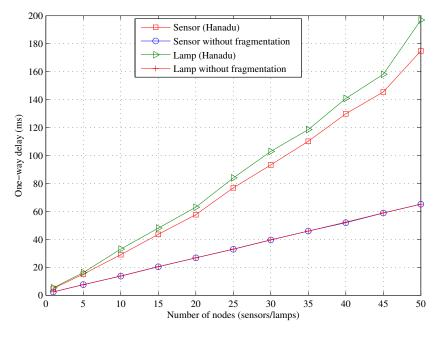
Figure 8. One-way delay for the sensor and lamp.
