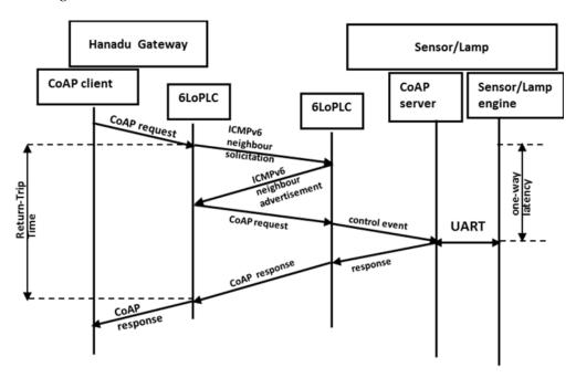
Figure 6. A schematic showing the end-to-end delay.
