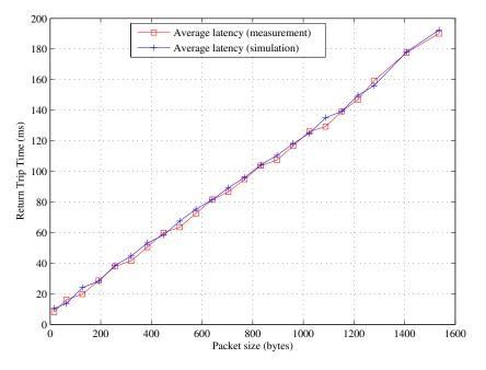
Figure 7. Model validation by comparing Return Trip Time (RTT) from simulation with measurement.
