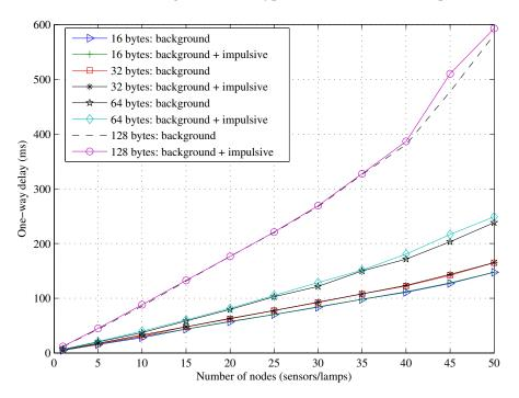
Figure 11. Effect of impulsive noise on one-way delay.
