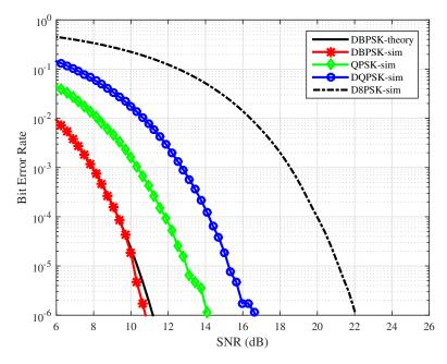
Figure 12. System Bit Error Rate (BER) performance as a function of Signal to Noise Ratio (SNR).
