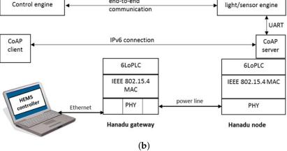
**Figure 1.** Hanadu low-power PLC system over the IPv6 network (6LoPLC) test bench showing (**a**) the main functional components and (**b**) the communication among system components.
