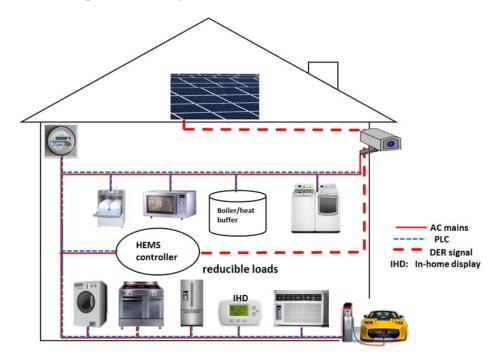
Figure 4. Home Energy Management System (HEMS) model showing various types of in-home loads.
