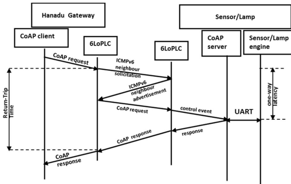
Figure 6. A schematic showing the end-to-end delay.
