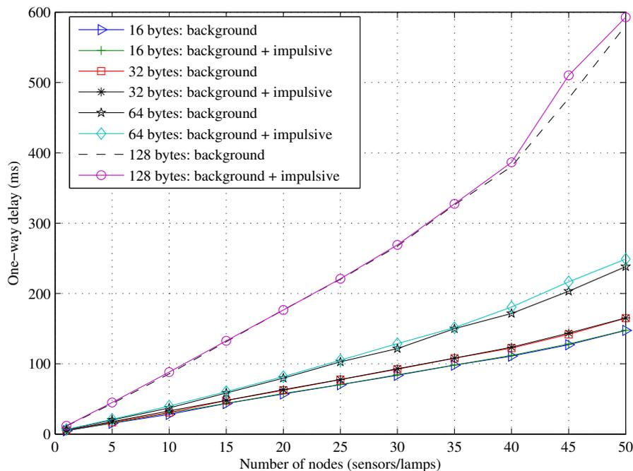
Figure 11. Effect of impulsive noise on one-way delay.
