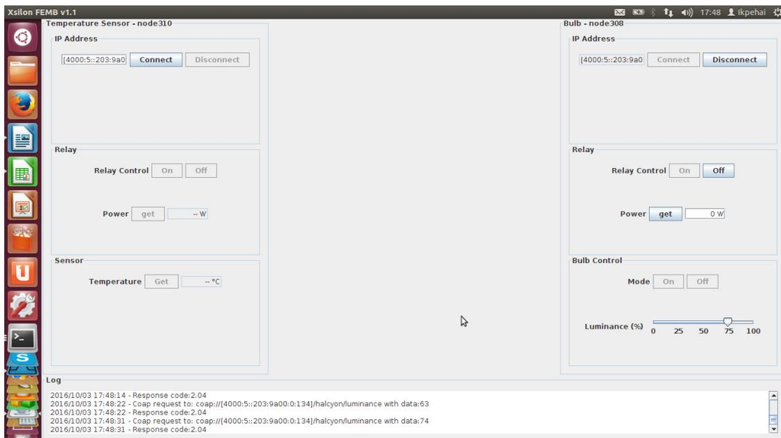
Figure 3. Constrained Application Protocol (CoAP) interface showing the monitoring (sensor) and control (lamp) windows.
