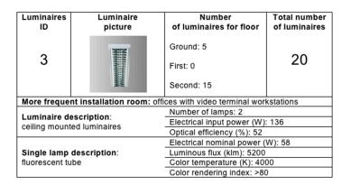
Figure 3. Example of the data collection sheet for a luminaire of the indoor lighting system.
