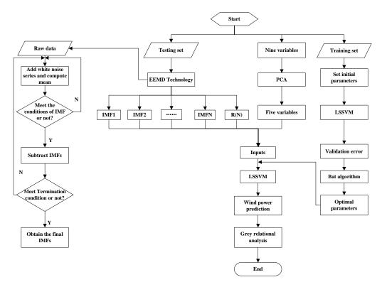
Figure 1. The flowchart of the proposed model.
