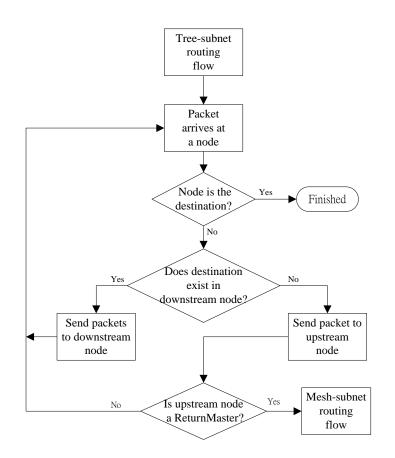
Figure 8. Tree-subnet routing flow diagram.
