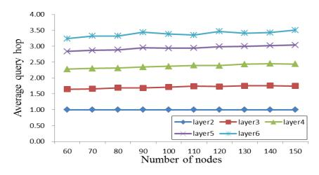
Figure 5. Average query hop in the mesh-shaped topology.
