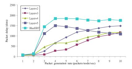
Figure 12. Average packet delay of mesh-tree and BlueHRT.
