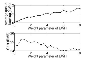
Figure 10. Average delay queue backlog of EWH and the electricity bills of controllable load.
