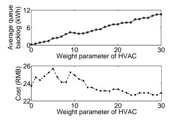
Figure 11. Average delay queue backlog of HVAC and the electricity bills of controllable load.
