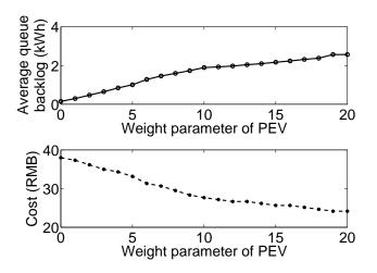
Figure 12. Average delay queue backlog of PEV and the electricity bills of controllable load.
