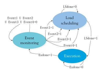
Figure 2. Diagram of the event-triggering mechanism.
