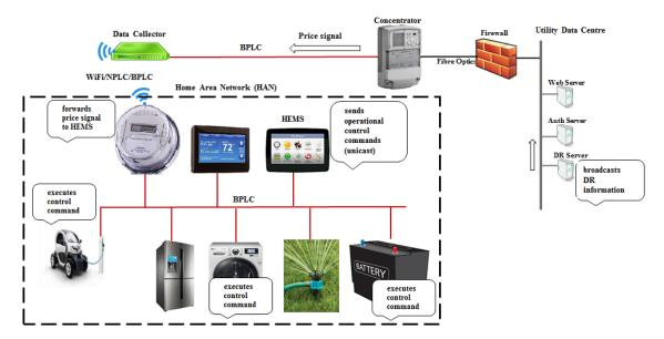
**Figure 2.** Transmission of peak price signal over the power line network.
