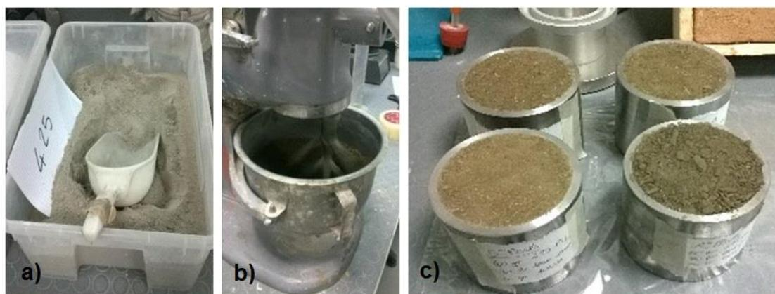
**Figure 5.** Mixing procedure of the mineralization process (a) Portland cement 4.25; (b) The material mixer; (c) The prepared samples and the moulds.
