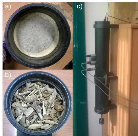
**Figure 9.** (a) Mineralized; (b) Unbound sample in the sample holder; and (c) Tube vertical configuration for the absorption analysis.
