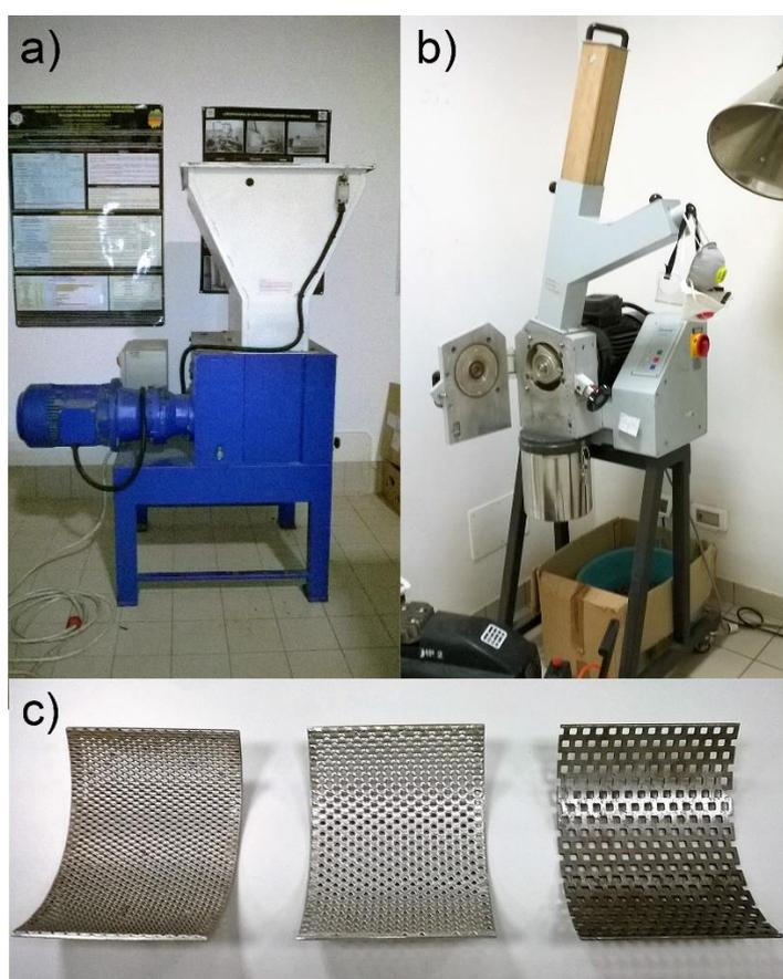
**Figure 2.** (a) Loose chips wood shredder; (b) Refining mill; (c) Refining mill grids.
