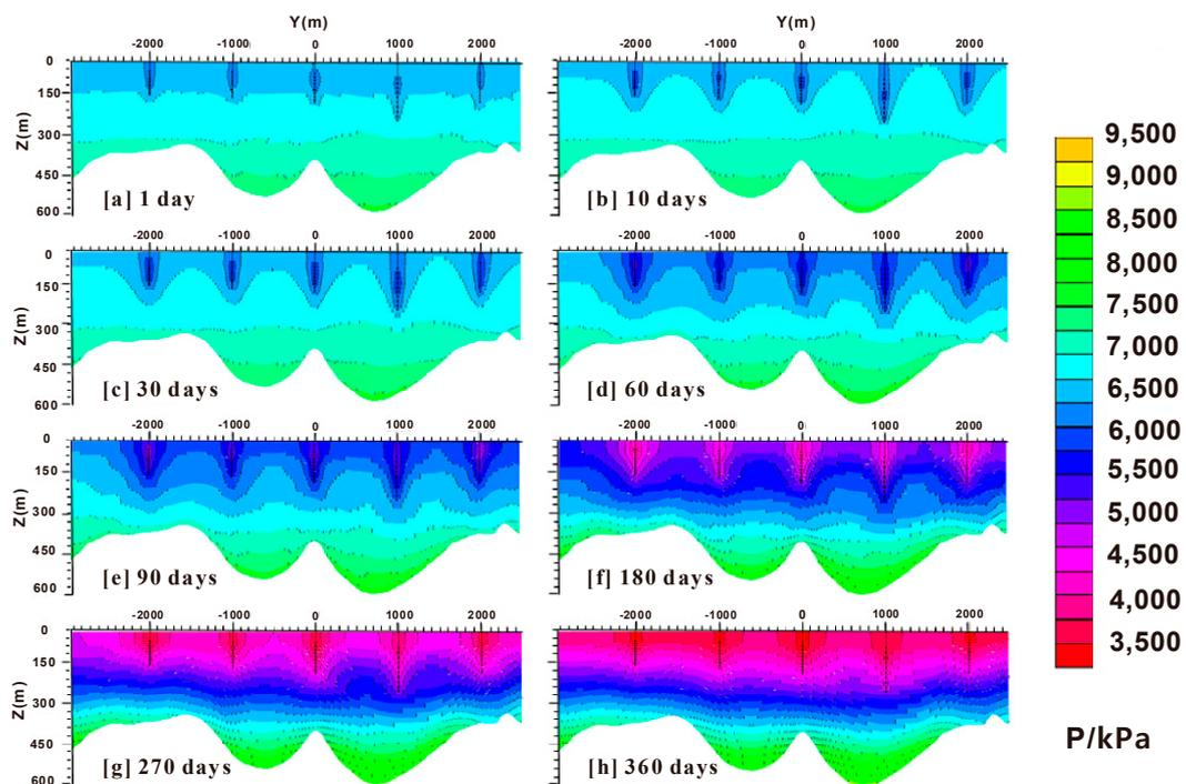
**Figure 10.** The evolution of spatial distribution of P during gas production from the methane hydrate deposit at some site of the Shenhu Area, South China Sea.
