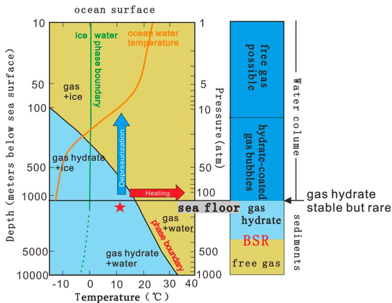
**Figure 3.** The mechanism for changing the pressure or the temperature conditions to destroy the stability of the original equilibrium and cause a phase change.
