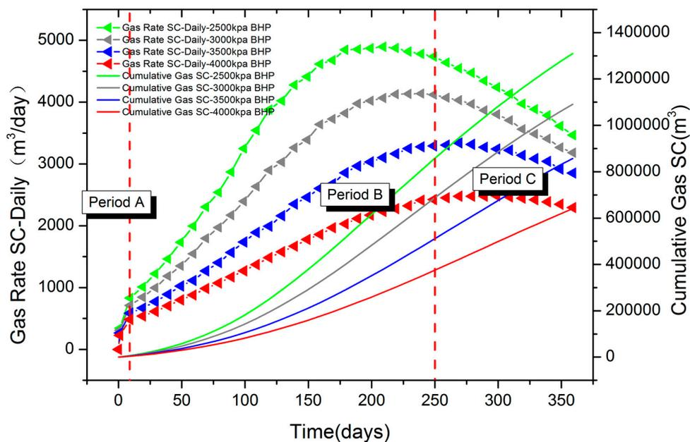
**Figure 12.** The volumetric rate of daily gas production and the cumulative gas production of four scenarios with different BHP in one years' simulation.
