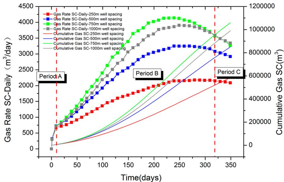
**Figure 11.** The volumetric rate of daily gas production and the cumulative gas production of four scenarios with different well spacing in one years' simulation.
