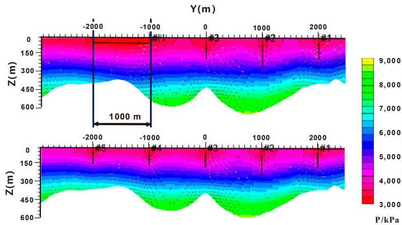
Figure 13. The pressure contrast of final moments with different well type.
