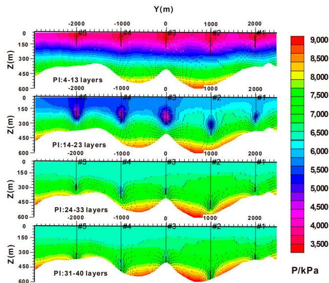
**Figure 16.** The pressure contrast of final moments with different perforation intervals.
