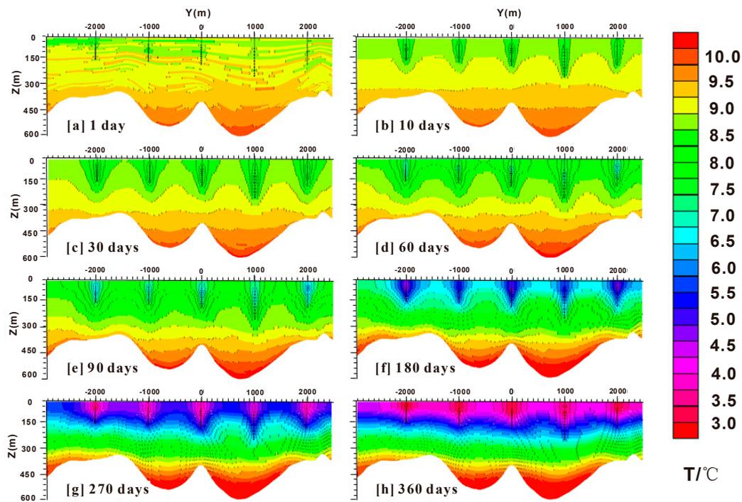
**Figure 9.** The evolution of spatial distribution of T during gas production from the methane hydrate deposit at some site of the Shenhu Area, South China Sea.
