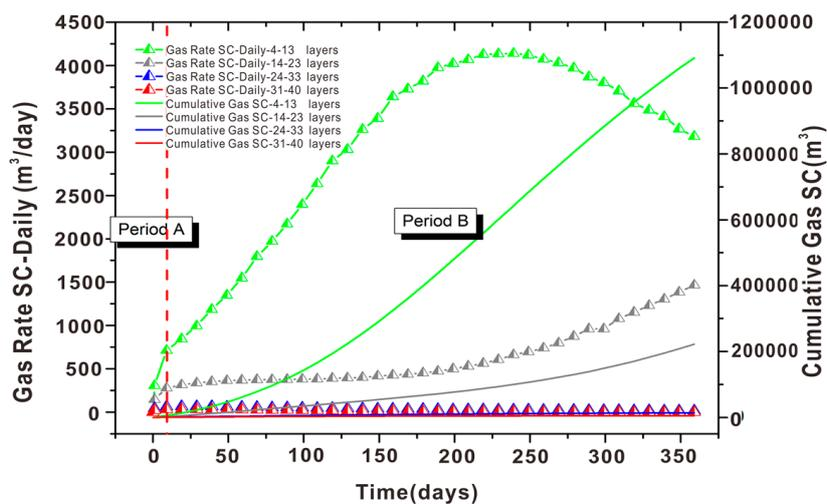
Figure 15. The volumetric rate of daily gas production and the cumulative gas production of two scenarios with different perforation intervals in one year's simulation.
