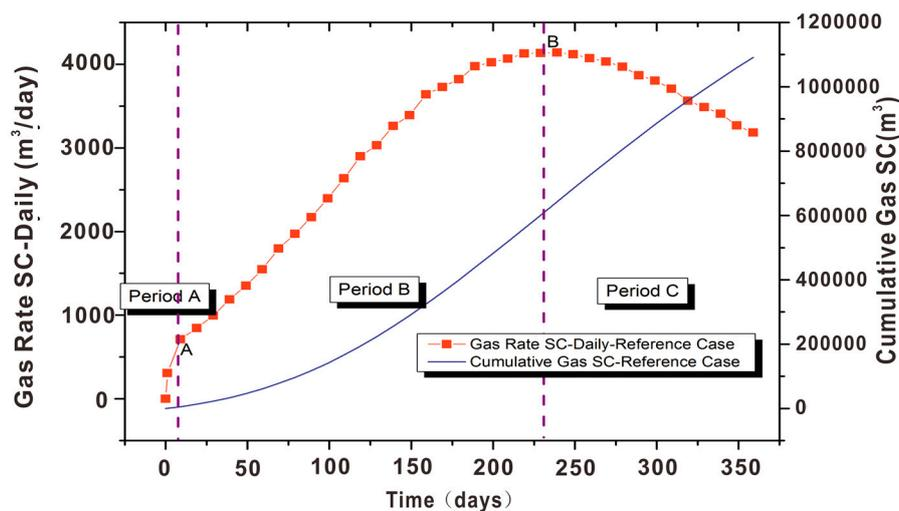
**Figure 6.** The volumetric rate of daily gas production and the cumulative gas production of reference case in one years' simulation.
