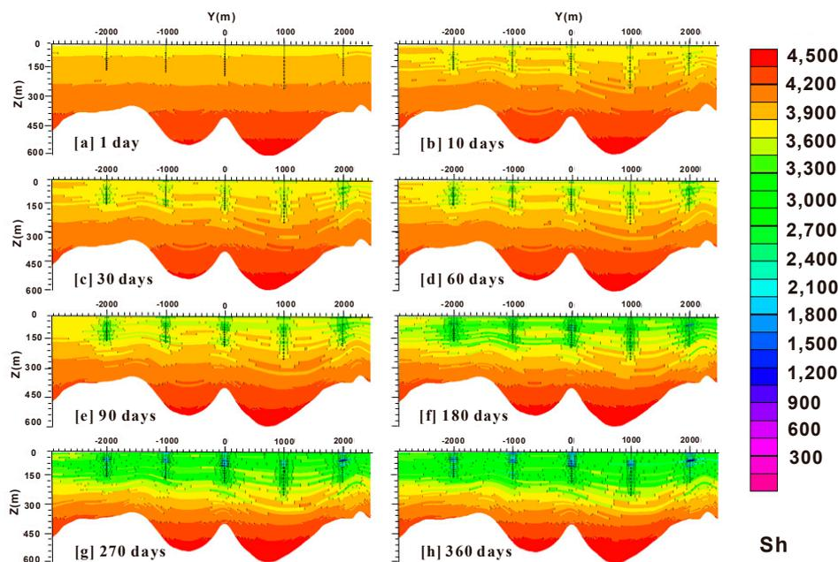
**Figure 8.** The evolution of spatial distribution of  $S_h$  during gas production from the methane hydrate deposit at some site of the Shenhu Area, South China Sea.
