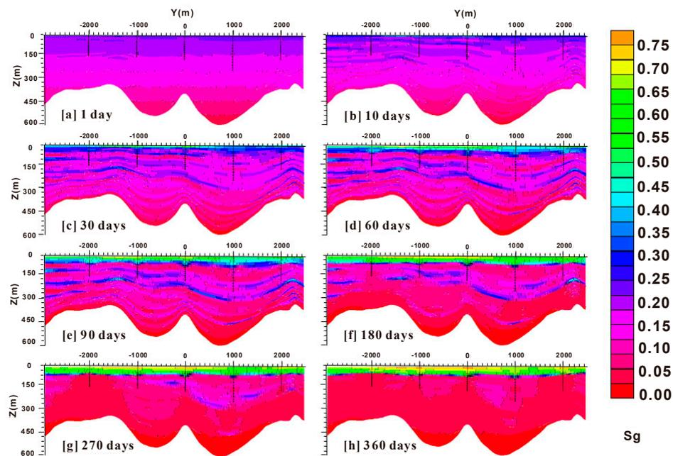
**Figure 7.** The evolution of spatial distribution of  $S_g$  during gas production from the methane hydrate deposit at some site of the Shenhu Area, South China Sea.
