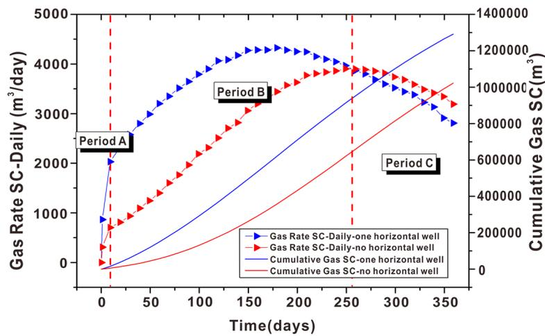
Figure 14. The volumetric rate of daily gas production and the cumulative gas production of two scenarios with different well type in one year's simulation.
