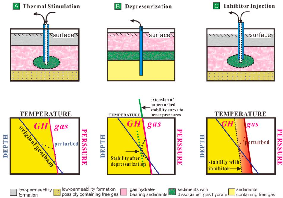
**Figure 2.** The mechanism of the three main methods to develop hydrate reservoirs. (A) Thermal Stimulation; (B) Depressurization; (C) Inhibitor Injection.
