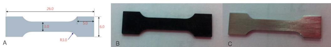
**Figure 1.** Magnesium (Mg) plate specimens. (A) Design of the magnesium plates; (B) Hydroxyapatite-coated magnesium plate (HA-Mg group); (C) Uncoated magnesium plate (Bare-Mg group).
