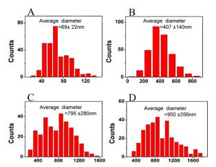
**Figure 2.** The fiber diameter distribution of zein (**A**); zein/gelatin-1 (**B**); zein/gelatin-2 (**C**); and zein/gelatin-3 (**D**) electrospun nanofibers.
