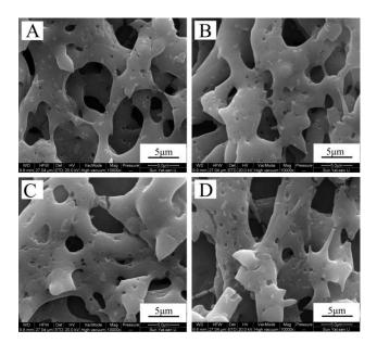
**Figure 4.** Morphological changes in zein (**A**); zein/gelatin-1 (**B**); zein/gelatin-2 (**C**); and zein/gelatin-3 (**D**) electrospun nanofibers after enzymatic degradation for 7 days.
