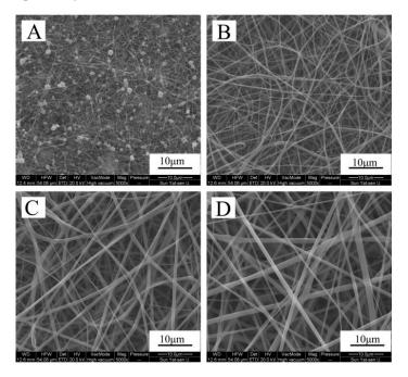
**Figure 1.** Scanning electron microscope (SEM) images of the surface morphology of zein (**A**); zein/gelatin-1 (**B**); zein/gelatin-2 (**C**); and zein/gelatin-3 (**D**) electrospun nanofibers.
