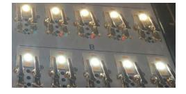
**Figure 3.** The CSP LED samples under 120 mA during the step-stress accelerated degradation test (SSADT) process. (Top: 4000 °K samples; Bottom: 5000 °K samples).
