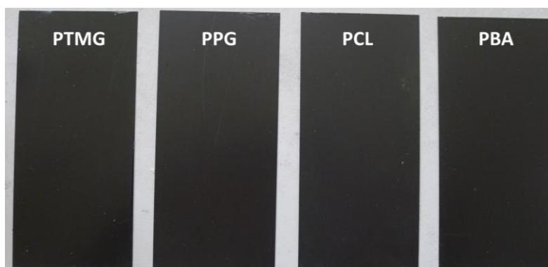
**Figure 8.** Black SDB-WPU coatings on the surface of steel plate with different soft segments: PTMG (polytetramethylene ether glycol); PPG (polypropylene glycol); PCL (polycaprolactone glycol); and PBA (poly-1, 4-butylene adipate glycol).
