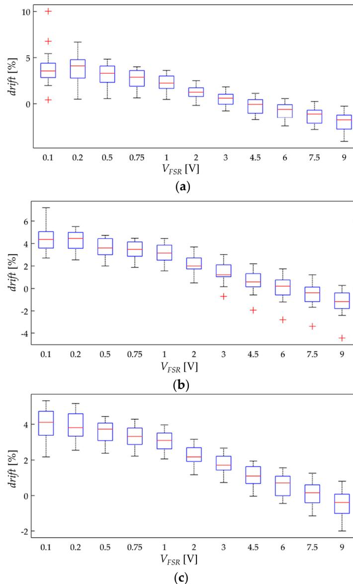
**Figure 10.** Box plots for the drift of sensor current after one hour of operation,  $drift(t = 3600 \text{ s})$ , when operating at multiple voltages,  $V_{FSR}$ . Drift data calculated from Equations (22) and (23) for sixteen FlexiForce A201-1 sensors at (a)  $\sigma = 42.1 \text{ KPa}$ , (b)  $\sigma = 105.4 \text{ KPa}$  and (c)  $\sigma = 210.8 \text{ KPa}$ .
