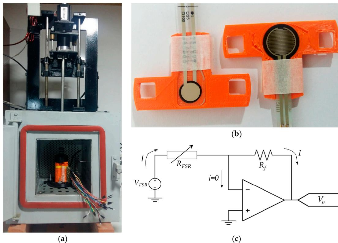
**Figure 9.** Test bench for gathering sensor data. (a) Overview of the mechanical set-up showing the load cell, the linear motor for the application of dynamic forces and the temperature chamber with the sixteen sensors in sandwich configuration. (b) Sensor holders for the FlexiForce A201-1 and Interlink FSR 402 sensors. (c) Amplifier in inverting configuration to drive each FSR with a constant voltage.
