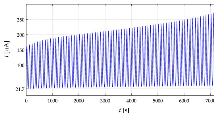
**Figure 15.** Simulation plot of sensor current,  $I(t)$ , when loaded to  $\sigma(t) = 200 \text{ KPa} + 100 \text{ KPa} \cdot \sin(2\pi 10^{-2} t)$  for two hours at  $V_{FSR} = 6 \text{ V}$ .
