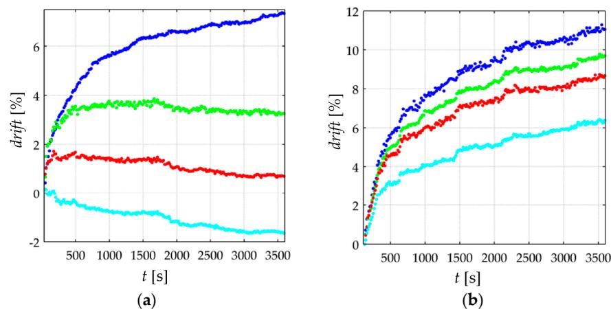
**Figure 12.** Time plots for the drift of sensor current calculated from Equation (22) at different voltages. Data taken for the (a) FlexiForce A201-1 sensor at  $\sigma = 210.8$  KPa for  $V_{FSR} = 1$  V (blue), 2 V (green), 6 V (red) and 9 V (cyan) and (b) Interlink FSR 402 sensor at  $\sigma = 65.6$  KPa for  $V_{FSR} = 0.2$  V (blue), 2 V (green), 3 V (red) and 7 V (cyan).
