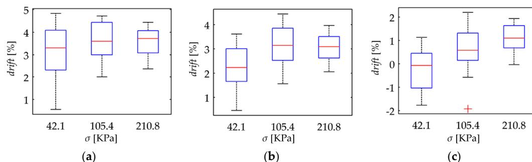
**Figure 13.** Box plots for the drift of sensor current after one hour of operation,  $drift(t = 3600 \text{ s})$ , when operating at different stresses,  $\sigma$ . Drift data calculated from Equations (22) and (23) for sixteen FlexiForce A201-1 sensors at (a)  $V_{FSR} = 0.5$  V, (b)  $V_{FSR} = 1$  V and (c)  $V_{FSR} = 4.5$  V.
