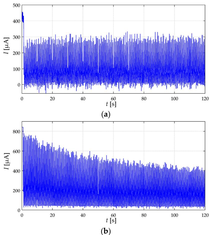
**Figure 16.** Experimental data taken for the A201-1 sensor when loaded to  $\sigma(t) = 115 \text{ KPa} + 95 \text{ KPa} \cdot \sin(4 \pi t)$  at (a)  $V_{FSR} = 2$  V and (b)  $V_{FSR} = 6$  V.
