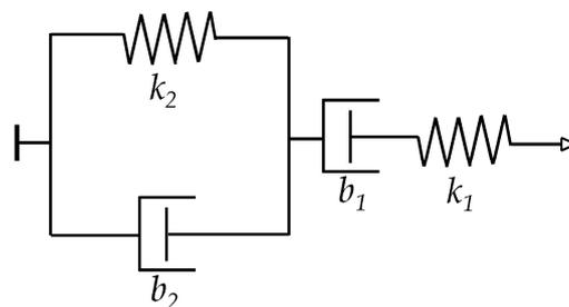
**Figure 5.** Generalized Burgers model [44] comprising two springs ( $k_1$ ,  $k_2$ ) and two dashpots ( $b_1$ ,  $b_2$ ).
