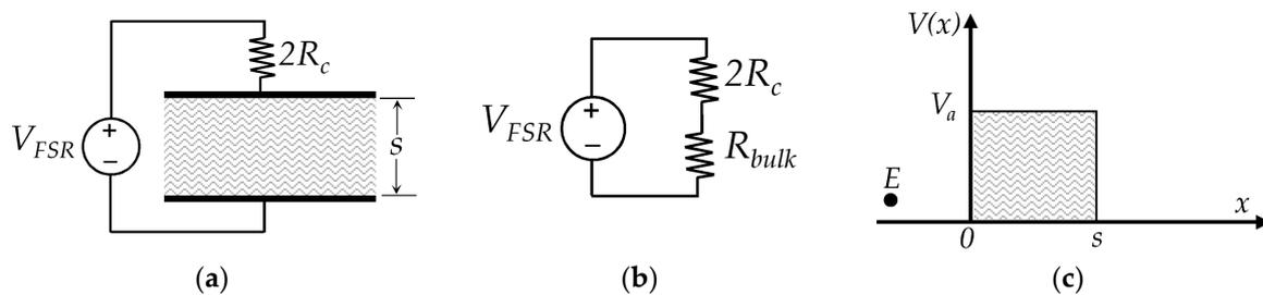
**Figure 2.** Elements and electrical model of a FSR connected to an external sourcing,  $V_{FSR}$ . (a) Series connection of a rectangular potential barrier with the contact resistance ( $R_c$ ), (b) Simplified sketch for the series connection between the contact resistance,  $R_c$ , and the bulk (tunneling) resistance,  $R_{bulk}$ . (c) Representation of a rectangular potential barrier with height  $V_a$  and width  $s$ . The particle shown is an electron with energy  $E$ .
