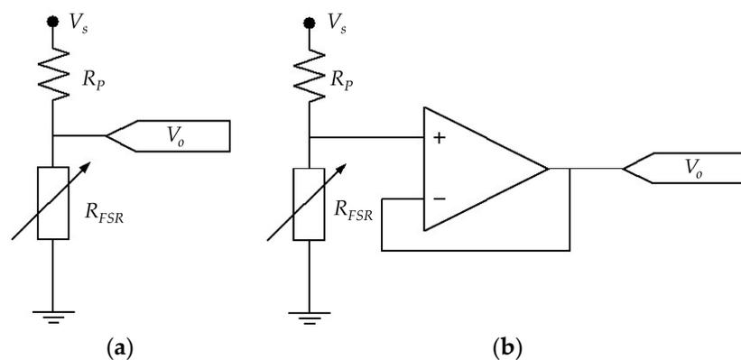
**Figure 17.** Voltage dividers for driving FSRs using (a) an unbuffered output and (b) a buffered output.
