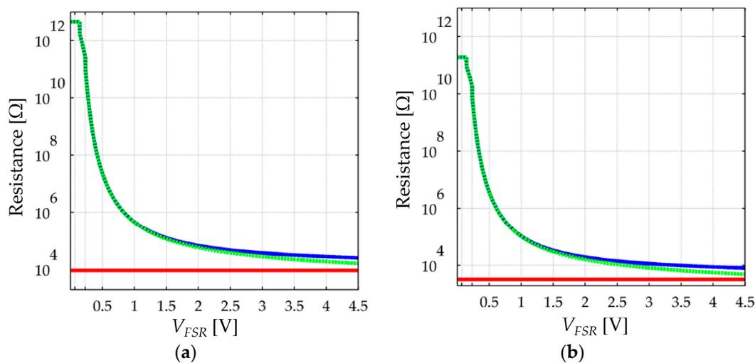
**Figure 8.** Simulation plots of the total resistance,  $R_{FSR}$  (blue), bulk resistance,  $R_{bulk}$  (green-dashed), and contact resistance,  $R_c$  (red), at two different stresses. (a)  $\sigma = 50$  KPa and (b)  $\sigma = 300$  KPa. Simulation done on the basis of Equations (9)–(11) using the parameters from Table 1 for the FlexiForce A201-1 sensor.
