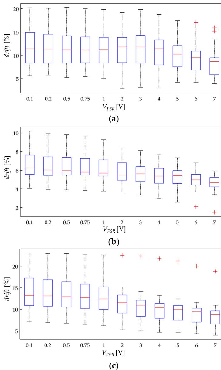
**Figure 11.** Box plots for the drift of sensor current after one hour of operation,  $drift(t = 3600 \text{ s})$ , when operating at multiple voltages,  $V_{FSR}$ . Drift data calculated from Equations (22) and (23) for sixteen Interlink FSR 402 sensors at (a)  $\sigma = 13.1 \text{ KPa}$ , (b)  $\sigma = 32.8 \text{ KPa}$  and (c)  $\sigma = 65.6 \text{ KPa}$ .
