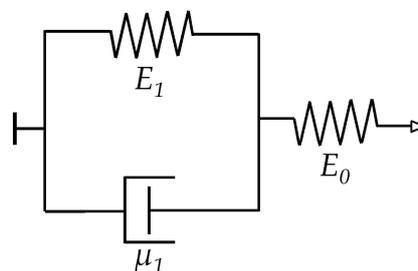
Figure 4. Rheological model for a Zener element [44] comprising two springs ( $E_0, E_1$ ) and a dashpot ( $\mu_1$ ).
