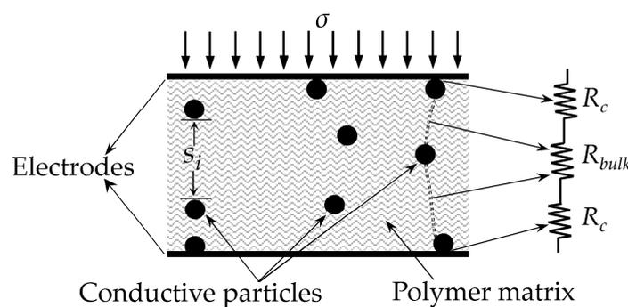
**Figure 1.** Sketch of a Conductive Polymer Composite (CPC) sandwiched between two metal electrodes to form a Force Sensing Resistor (FSR). The electrical model of the FSR comprises a series connection between the bulk (tunneling) resistance ( $R_{bulk}$ ) and the contact resistance ( $R_c$ ).
