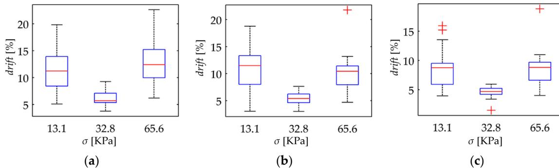
**Figure 14.** Box plots for the drift of sensor current after one hour of operation,  $drift(t = 3600 \text{ s})$ , when operating at different stresses,  $\sigma$ . Drift data calculated from Equations (22) and (23) for sixteen Interlink FSR 402 sensors at (a)  $V_{FSR} = 1 \text{ V}$ , (b)  $V_{FSR} = 4 \text{ V}$  and (c)  $V_{FSR} = 7 \text{ V}$ .
