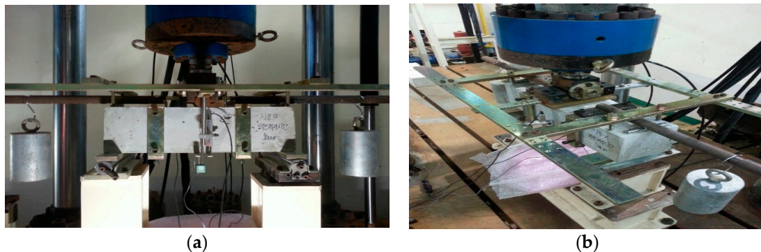
Figure 6. Three-point bending test set-up: (a) Front view; (b) Top perspective view
