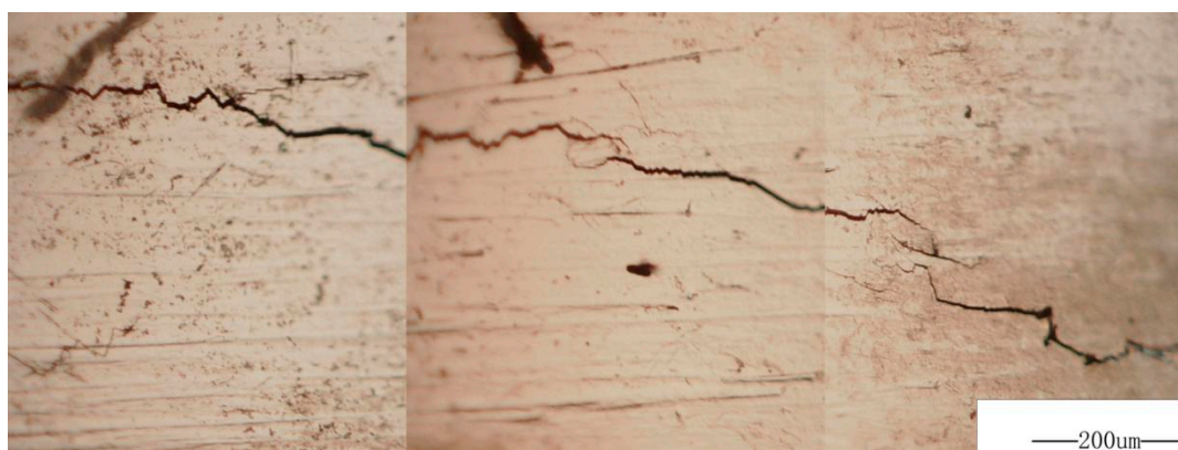
Figure 15. Morphology of fatigue precracks propagation.
