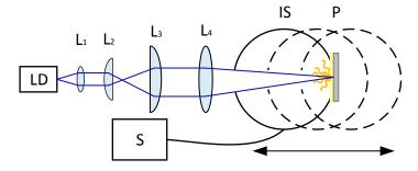
**Figure 7.** Optical scheme of the PC-LD setup. IS is an integrating sphere and S is a spectrometer. The integrating sphere, including the phosphor and temperature controlled substrate, can be translated.
