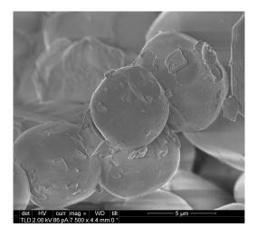
Figure 6. SEM images of the phosphor material used for the PC-LD light source.
