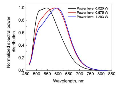
Figure 2. Normalized measured spectral power distribution of the phosphor emision at three different input laser powers for a laser spot diameter of 337  $\mu m$ .
