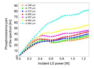
Figure 4. Integrated downconverted luminous flux vs input laser power at several laser spot diameters.
