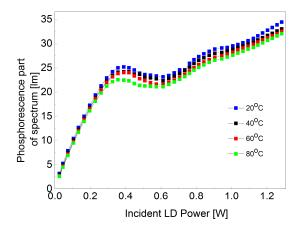
**Figure 5.** Integrated downconverted luminous flux vs input laser power at different phosphor aluminum substrate temperatures at 190  $\mu$ m spot size diameter.
