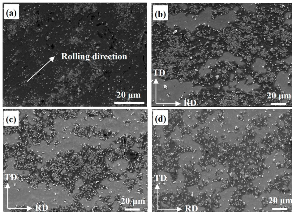
**Figure 3.** Microstructures of Al-TiB<sub>2</sub>/TiC in situ composites with different deformation processes (in RD-TD plane). (a) Rolling for 90% reduction; (b–d) Following one, two and four ARB cycles, respectively.
