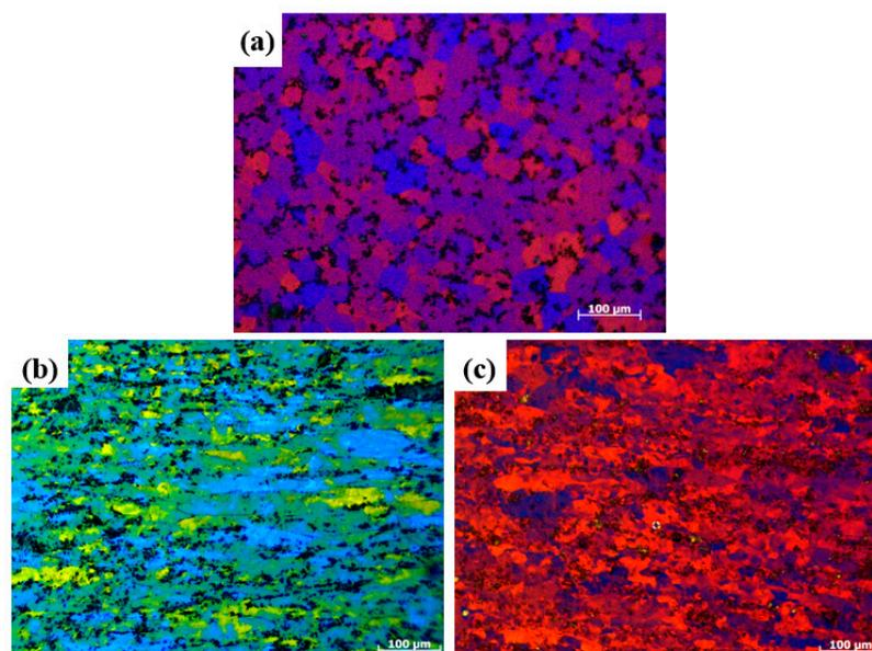
**Figure 6.** Polarized light optical micrograph of Al-TiB<sub>2</sub>/TiC in situ composites: (a) As cast; (b) Rolled for 90% reduction; (c) After one ARB cycle.
