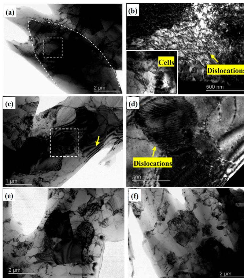
**Figure 7.** Typical TEM micrographs of Al-5 wt % TiB<sub>2</sub>/TiC composites: (a,b) After rolling for 90% reduction; (c,d) After one ARB cycle; (e) After two ARB cycles; (f) After four ARB cycles.
