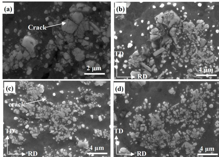
**Figure 4.** Effect of deformation on the particle distribution of the composites in the RD-TD plane. (a) Rolling for 90% reduction; (b–d) Following one, two and four ARB cycles, respectively.
