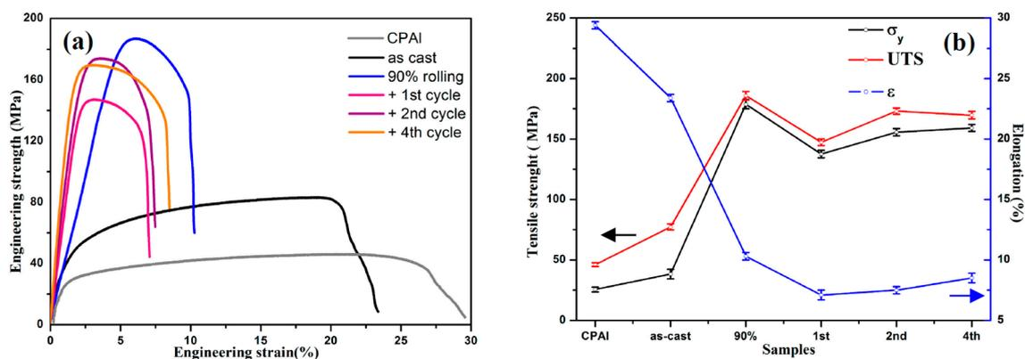
**Figure 8.** Tensile properties of the Al-TiB<sub>2</sub>/TiC composites. (a) Typical engineering stress-strain curves of the composites and CPAI; (b) Variations of  $\sigma_y$ , UTS and elongation of the composites as a function of different deformation treatments.
