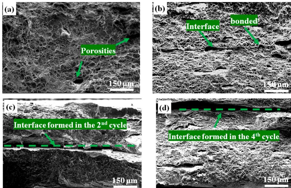
**Figure 9.** Tensile fracture surfaces of the Al-TiB<sub>2</sub>/TiC composites: (a) As cast; (b–d) After one, two and four ARB cycles, respectively.
