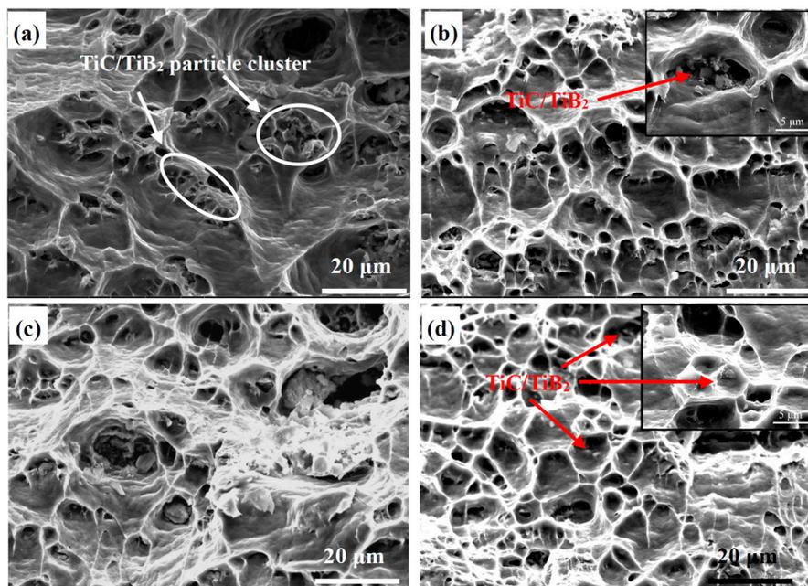
**Figure 10.** Fractography of Al-TiB<sub>2</sub>/TiC composites at higher magnification: (a) As cast; (b–d) After one, two and four ARB cycles, respectively.
