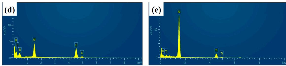
**Figure 2.** XRD pattern and FESEM micrographs of Al-TiB<sub>2</sub>/TiC in situ composites: (a) XRD pattern; (b,c) Microstructures at low and high magnification; (d,e) EDS point analysis for the particles.
