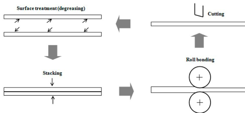
Figure 1. Diagrammatic illustration of the accumulative roll-bonding (ARB) process.
