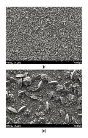
Figure 4. Surface morphology of the BiTe deposition potentials: (a) -40 mV; (b) 20 mV; and (c) 60 mV.
