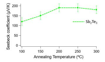
Figure 21. Dependence of the Seebeck coefficients from the Sb<sub>2</sub>Te<sub>3</sub> on the annealing temperature.
