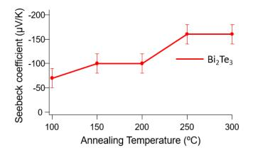
Figure 15. Dependence of the Seebeck coefficients on the annealing temperature.
