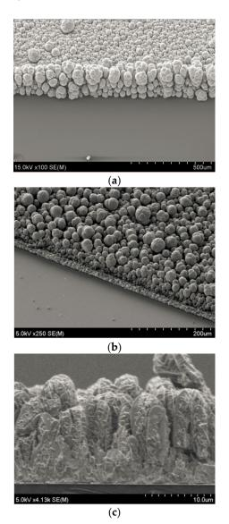
**Figure 8.** Morphology of the thick BiTe film synthesized by the constant potential method: (a) 200-µm-thick film; (b) cross-section view of the 200-µm-thick film consisting of two different layers; and (c) cross-section structure of the initial 10-µm-thick film.
