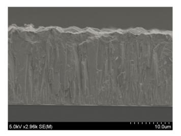
Figure 11. Cross-section structure of the film grown by pulsed deposition.
