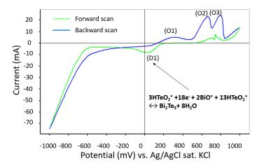
Figure 2. Cyclic voltammetry for BiTe deposition.
