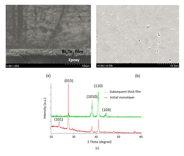
**Figure 6.** The dependence of the metallic seed layer on the lattice matching of the initial monolayer: (a) sample structure after being separated from the metallic seed layer with the monolayer on the top surface; (b) surface morphology determined via Scanning Electron Microscopy (SEM) observation; and (c) XRD pattern of the initial monolayer.
