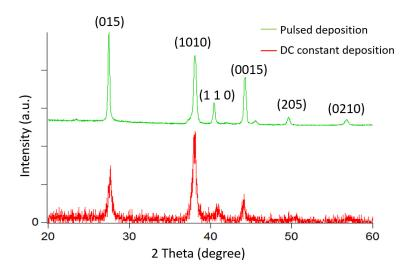
Figure 19. XRD patterns of the  $Sb_2Te_3$  films synthesized by constant and pulsed deposition at -144 mV.
