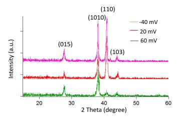
Figure 5. X-ray diffraction (XRD) pattern of the BiTe films for different deposited potentials.
