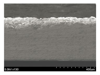
Figure 18. SEM image of the cross section of the 500-µm-thick Sb<sub>2</sub>Te<sub>3</sub> film.
