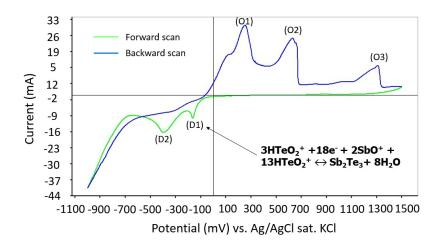
Figure 16. Cyclic voltammetry of SbTe deposition.
