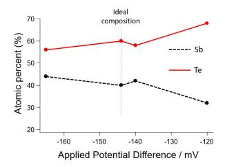
**Figure 17.** Potentials dependence on the atomic composition of the Sb<sub>2</sub>Te<sub>3</sub>.
