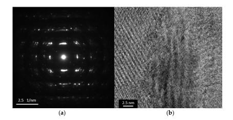
**Figure 7.** (a) Selected Area Electron Diffraction (SAED) pattern; and (b) High Resolution Transmission Electron Microscopy (HRTEM) observation between the boundaries of the Bi<sub>2</sub>Te<sub>3</sub> sample.
