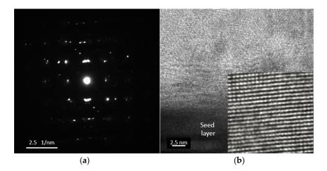
**Figure 14.** (**a**) SAED pattern; and (**b**) HRTEM observation between the boundaries of the Bi<sub>2</sub>Te<sub>3</sub> sample fabricated using pulsed deposition.
