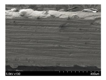
Figure 12. SEM image of the cross section of the 600-µm-thick Bi<sub>2</sub>Te<sub>3</sub> film.
