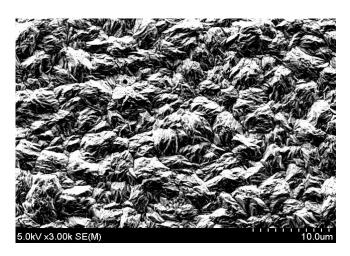
Figure 10. SEM image of Bi<sub>2</sub>Te<sub>3</sub> film surface formed by pulsed deposition.
