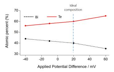
Figure 3. Potential dependence on the atomic composition of BiTe.
