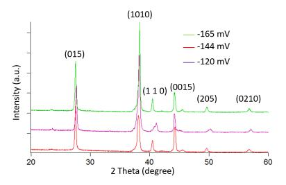
Figure 20. XRD pattern of the SbTe films at different deposited potentials.
