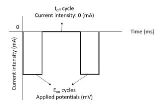
Figure 9. Pulsed deposition waveform.
