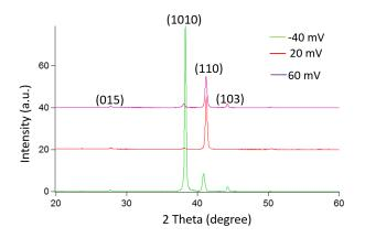
Figure 13. XRD pattern of the BiTe films with different deposited potentials.
