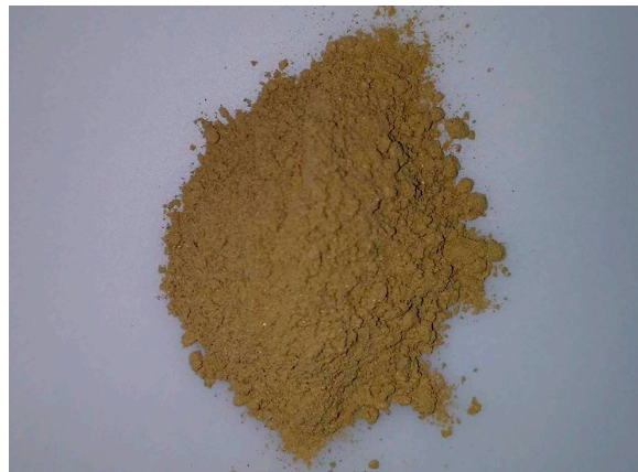
Figure 2. Sand washing waste used as filler for epoxy resin mortar in this study.
