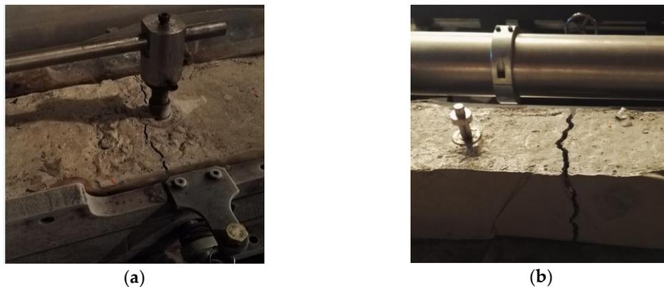
**Figure 12.** The failure patterns with different deformation measurement methods. (a) The sample with top, left, and right embedded parts in Section 3.1. (b) The sample with top embedded part in Section 3.3.
