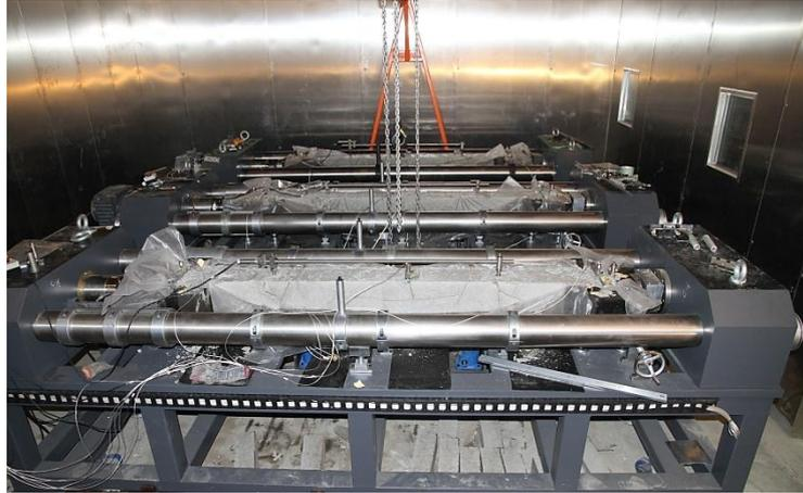
**Figure 9.** TSTM after the demolding.
