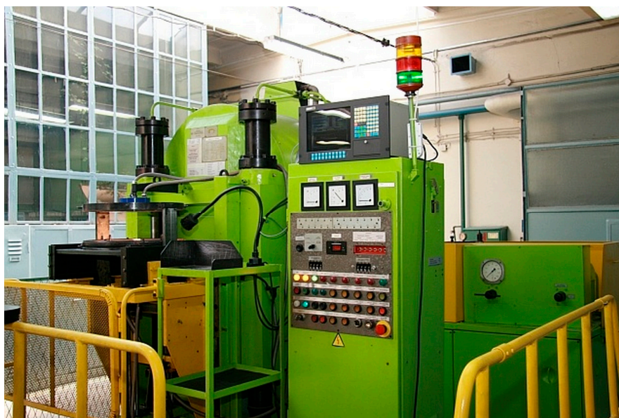
Figure 1. High-pressure spark plasma sintering (HP SPS) apparatus in the Institute of Advanced Manufacturing Technology, Krakow.
