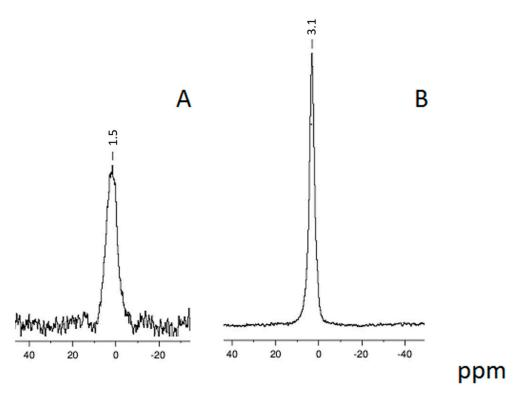
Figure S4. Typical 31P NMR spectra of CSCaP (A) and CSCaPC (B) samples.
