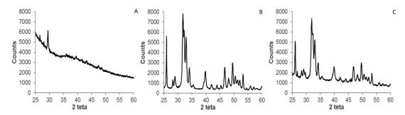
**Figure S2.** XRD pattern of **(A)** chitosan, **(B)** hydroxyapatite and **(C)** physical mixture of chitosan and hydroxyapatite.
