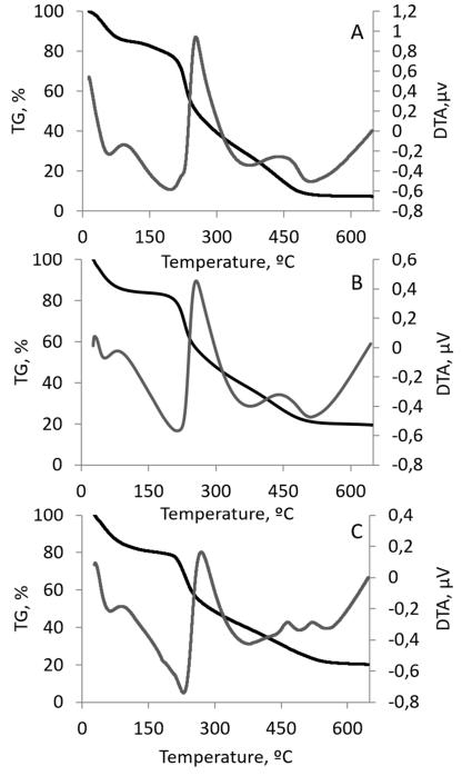
**Figure S1.** Thermogavimetric analysis of CSCaP composites. **(A)** CSCaP1, **(B)** CSCaP2 and **(C)** CSCaP3 samples.
