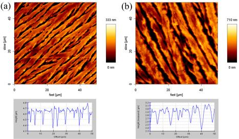
**Figure 1.** Atomic force microscopy (AFM) images (50  $\mu$ m  $\times$  50  $\mu$ m) and cross-section height profiles at: (a) 2 mM; and (b) 8.1 mM.
