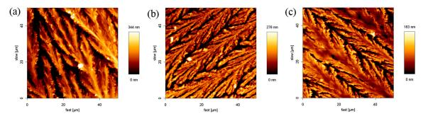
**Figure 4.** AFM images of SDS-inorganic salt aggregates on the surface of the glass: (**a**) SDS-NaCl; (**b**) SDS-NaI; and (**c**) SDS-NaNO<sub>2</sub>.
