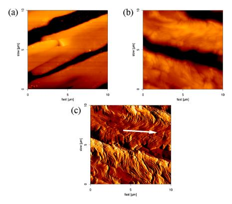
**Figure 2.** AFM images (10  $\mu$ m  $\times$  10  $\mu$ m) (**a**) at 2 mM and (**b**) at 8.1 mM; and (**c**) AFM error signal image from (b).
