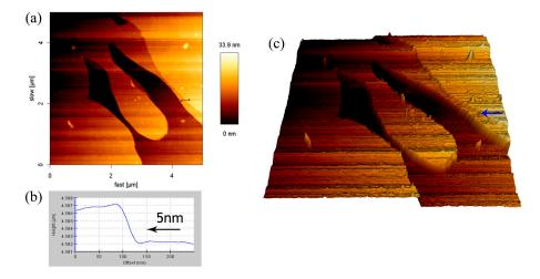
**Figure 7.** AFM result of SDS-CsCl aggregates of the surface of the glass: (**a**) height image; (**b**) cross-section height profiles along the line in (a); and (**c**) 3D reconstruction image.
