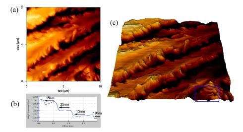
**Figure 6.** AFM result of SDS-NaCl aggregates of the surface of the glass: (**a**) height image; (**b**) cross-section height profiles along the line in (a); and (**c**) 3D reconstruction image.
