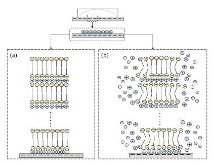
**Figure 8.** Schematic representation of possible mechanisms for surfactant adsorption on a glass slide: (a) SDS; and (b) SDS-monovalent ions.
