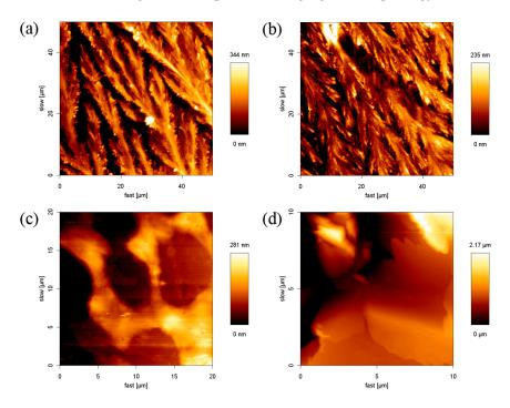
**Figure 3.** AFM images of SDS-inorganic salt aggregates on the surface of the glass: (**a**) SDS-NaCl; (**b**) SDS-KCl; (**c**) SDS-MgCl<sub>2</sub>; and (**d**) SDS-CaCl<sub>2</sub>.
