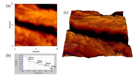
**Figure 5.** AFM result of SDS aggregates of the surface of the glass: (**a**) height image; (**b**) cross-section height profiles along the line in (**a**); and (**c**) 3D reconstruction image.
