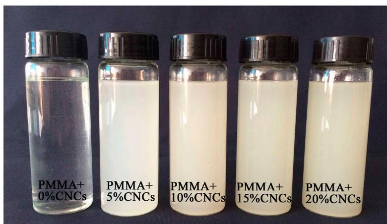
Figure 4. Photograph of pure PMMA solutions and PMMA + CNCs suspensions.
