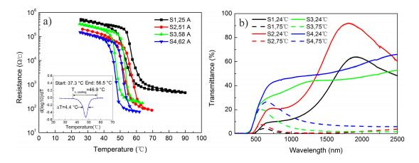
**Figure 2.** (**a**) Temperature dependencies of the electrical resistance for the as-deposited VO<sub>2</sub> thin films; and (**b**) the transmittance spectra of the as-deposited VO<sub>2</sub> films at various temperatures.
