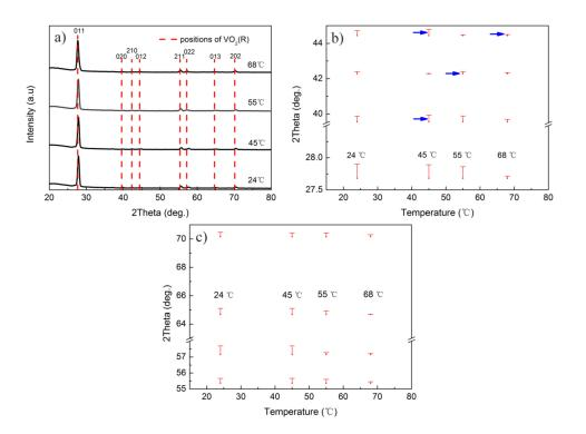
**Figure 8.** (a) XRD patterns of sample S2 during the heating processes; and (**b**,**c**) magnified 2 $\theta$  differences between the experimental diffraction angles and those of the standard VO<sub>2</sub>(R) at different temperatures. Therein, the diffraction angles indicated by the blue arrows increased instead of decreasing during heating process.
