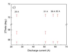
**Figure 3.** (a) X-ray diffraction (XRD) patterns of the as-deposited VO<sub>2</sub> thin films grown on quartz substrates; and (**b**,**c**) the magnified 2 $\theta$  differences between the experimental diffraction angles of the as-deposited films and those of the standard VO<sub>2</sub>(R).
