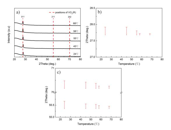
**Figure 7.** (a) XRD patterns of sample S4 during the heating process, and (**b**,**c**) magnified 2 $\theta$  differences between the experimental diffraction angles and those of the standard VO<sub>2</sub>(R) at different temperatures.
