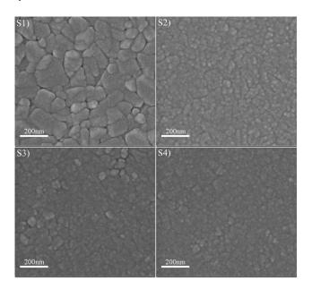
Figure 5. Scanning electron microscope (SEM) images of as-deposited VO<sub>2</sub> thin films.
