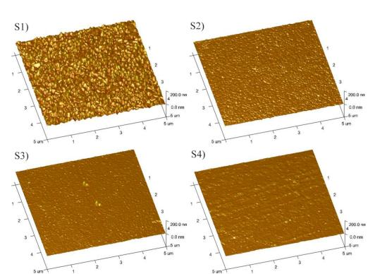
Figure 6. Atomic force microscope (AFM) images of as-deposited VO<sub>2</sub> thin films.
