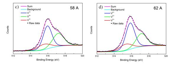
**Figure 4.** X-ray photoelectron spectroscopy (XPS) V(2P) spectra for different as-deposited VO<sub>2</sub> thin films. (**a**) S1; (**b**) S2; (**c**) S3; and (**d**) S4.
