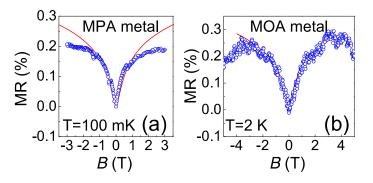
**Figure 5.** Positive MR in metallic devices. (a) an MPA metallic device in the parallel field at  $T \sim 100$  mK; (b) an MOA metallic device in the perpendicular field at T = 2 K. Red curves are fitting results by using Equations (11) and (12).
