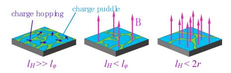
**Figure 7.** The formation of charge puddles in the AI and charge hopping between them. The red arrows show the perpendicular magnetic fields *B*. At the intermediate magnetic field  $l_H < \sim l_{\phi}$ , the size of the charge puddles becomes enlarged. When the field is so large that  $l_H < 2r$ , the quantum interference is totally destroyed.
