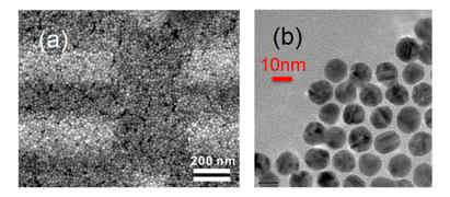
**Figure 1.** (a) the scanning electron micrograph of a 8-mercaptooctanoic acid (MOA) device; rectangles with a light color are the measurement electrodes; (b) the transmission electron microscopy image of the synthesized Au nanoparticles deposited on a  $Si_3N_4$  membrane. Here, the capping molecules are 11-mercaptoundecanoic acid (MUA) molecules.
