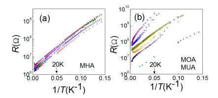
**Figure 3.** *R* vs. 1/T plots for insulating MHA (**a**), MOA and MUA (**b**) devices. Each color represents individual device. At higher temperatures, the resistance follows the thermal activation property, namely,  $\ln R \sim T^{-1}$ . There is a slight deviation near room temperature, suggesting effect from thermal expansion.
