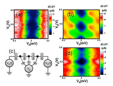
**Figure 9.** (a) the experimental data of dynamical conductance for a different MPA AI device; (b) the calculated dynamical conductance of a single-island SET circuit; (c,d) the assumed three-island circuit and calculated dynamical conductance.
