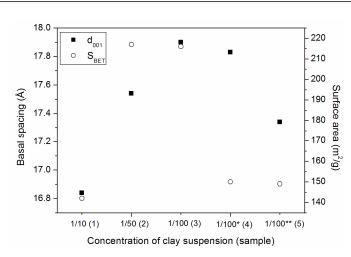
**Figure 2.** Relation between the concentration of the clay suspension to basal space (Å) and surface area BET  $(m^2/g)$  for series 1 samples. \* 500 mL and \*\* 900 mL of water removed before pilarization.
