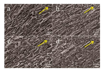
**Figure 4.** SEM images of the freeze-fractured cross-section surfaces of **(a)** BNNSs/PVDF; **(b)** BNNSs@C-5/PVDF; **(c)** BNNSs@C-15/PVDF; and **(d)** BNNSs@C-45/PVDF nanocomposites at 20 vol % filler loadings.
