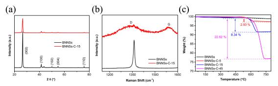
**Figure 3.** (a) XRD patterns; (b) Raman spectra; and (c) TGA curves of pristine BNNSs and corresponding BNNSs@C hybrids with different CVD deposition times.
