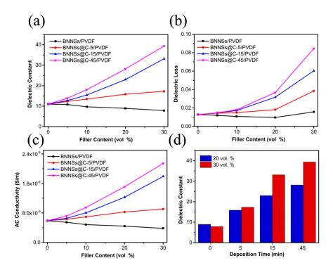
**Figure 6.** Dependence of the (**a**) dielectric constant; (**b**) dielectric loss; and (**c**) ac conductivity values of BNNSs/PVDF, BNNSs@C-5/PVDF, BNNSs@C-15/PVDF, and BNNSs@C-45/PVDF nanocomposites on the filler loadings (10<sup>3</sup> Hz); (**d**) Typical variation of dielectric constant values (10<sup>3</sup> Hz) of BNNSs/PVDF and BNNSs@C/PVDF nanocomposites as a function of carbon deposition time at different filler loadings (20 and 30 vol %).
