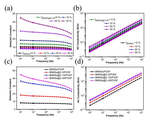
**Figure 5.** Frequency dependence of the **(a)** dielectric constant and **(b)** ac conductivity values of BNNSs/PVDF and BNNSs@C-45/PVDF nanocomposites at different filler loadings; Typical frequency-dependent comparison of **(c)** dielectric constant and **(d)** ac conductivity values of BNNSs/PVDF, BNNSs@C-5/PVDF, BNNSs@C-15/PVDF, and BNNSs@C-45/PVDF nanocomposites at equivalent filler loadings (30 vol %).
