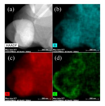
**Figure 2.** (a) HAADF-STEM image of the BNNSs@C-15 hybrids; (b-d) EDX elemental maps of B, N, and C, respectively.
