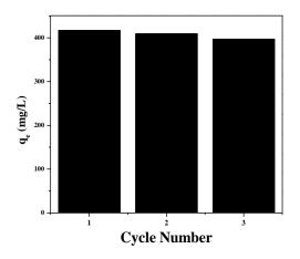
Figure 9. Eluting regeneration cycles and adsorption capacity.
