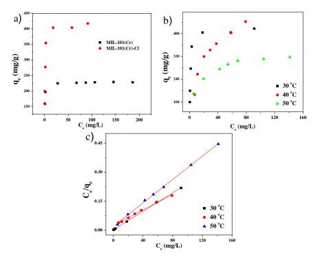
**Figure 7.** (a) Standard adsorption curves for 2,4-D on MIL-101(Cr) (black line) and MIL-101(Cr)-Cl (red line) at 30 °C; (b) adsorption isotherms for MG on MIL-101(Cr)-Cl at different temperatures; and (c) Langmuir plots of the isotherms for the adsorption of 2,4-D adsorption onto MIL-101(Cr)-Cl.
