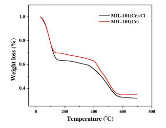
Figure 4. TGA graph of MIL-101(Cr) (red line) and MIL-101(Cr)-Cl (black line).
