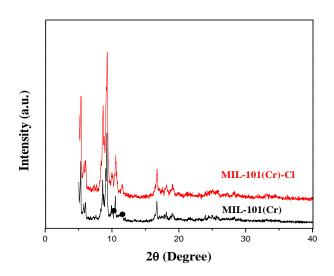
Figure 1. Powder X-ray diffraction (PXRD) patterns of MIL-101(Cr) and MIL-101(Cr)-Cl.
