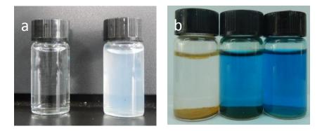
**Figure 5.** (a) Left is the supernatant liquid of MIL-101(Cr)-Cl soaked in water with added AgNO<sub>3</sub> solution, right is the supernatant liquid of MIL-101(Cr)-Cl soaked in NaNO<sub>3</sub> solution with added AgNO<sub>3</sub> solution; (b) Left is methyl orange (MO) after adsorption by MIL-101(Cr)-Cl, middle is MO + MB after adsorption by MIL-101(Cr)-Cl, and right is MB after adsorption by MIL-101(Cr)-Cl.
