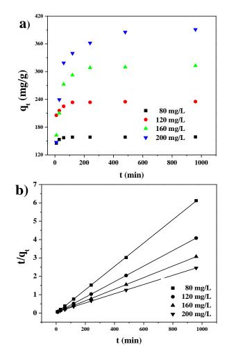
**Figure 6.** (a) Effect of contact time on the adsorption of 2,4-D on MIL-101(Cr)-Cl (10 mg) at different initial concentrations of 2,4-D at 30 °C; (b) Plots of pseudo-second-order kinetics for the adsorption of 2,4-D at 30 °C.
