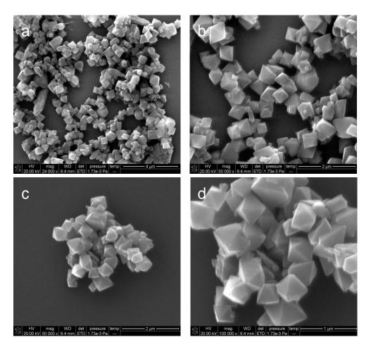
Figure 3. SEM images of MIL-101(Cr) (a,b) and MIL-101(Cr)-Cl (c,d).
