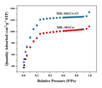
Figure 2. N2 adsorption-desorption isotherms of as-synthesized MIL-101(Cr) and MIL-101(Cr)-Cl.
